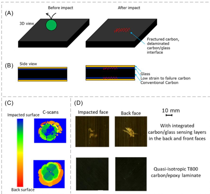
**Figure 2.6** Visual inspection of barely visible impact damage in self-reporting composites by means of hybrid carbon/glass coatings: (A) schematic 3D view, (B) schematic side view of the substrate and the integrated sensor, (C) C-scan results, and (D) impacted face and back face images of specimens with (up) and without (bottom) carbon/glass coating.
