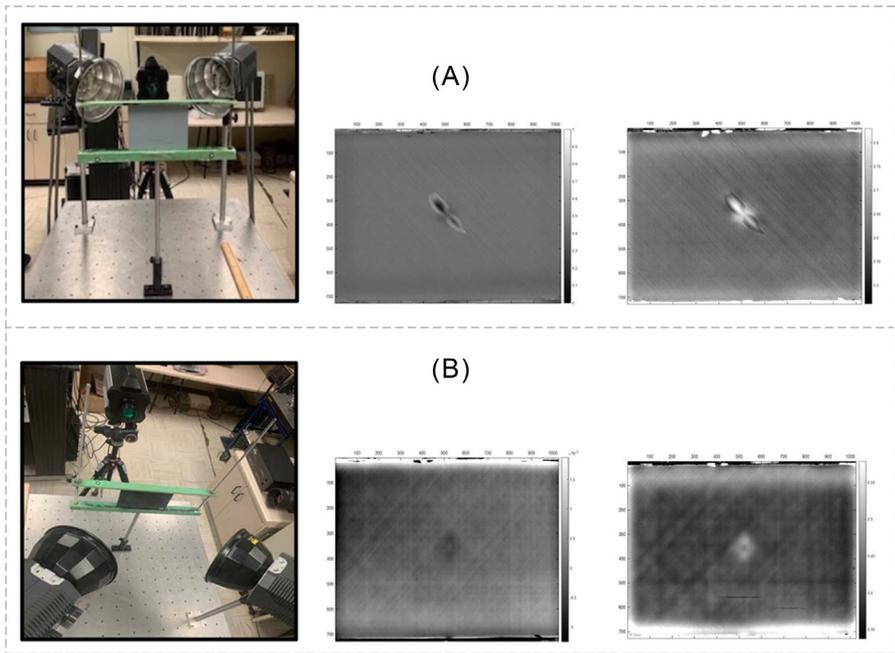
**Figure 2.7** Methods for image capture presented in Alhammad et al. (2022). Reflect mode (A) captures the image from the impacted side and transmission mode (B) captures images of the nonimpacted side.
