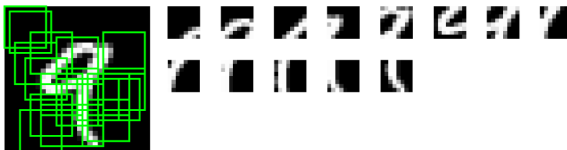
Figure C.5: The thirteen instances generated by taking twenty random patches from an MNIST image. On the left, an example image of a handwritten nine is shown, with the patches plotted on the number. All smaller pictures on the right are the generated instances from these patches. Only thirteen instances are generated because the other instances contain an average gray-scale value below the cut-off point. The cut-off instances are almost entirely dark squares.
