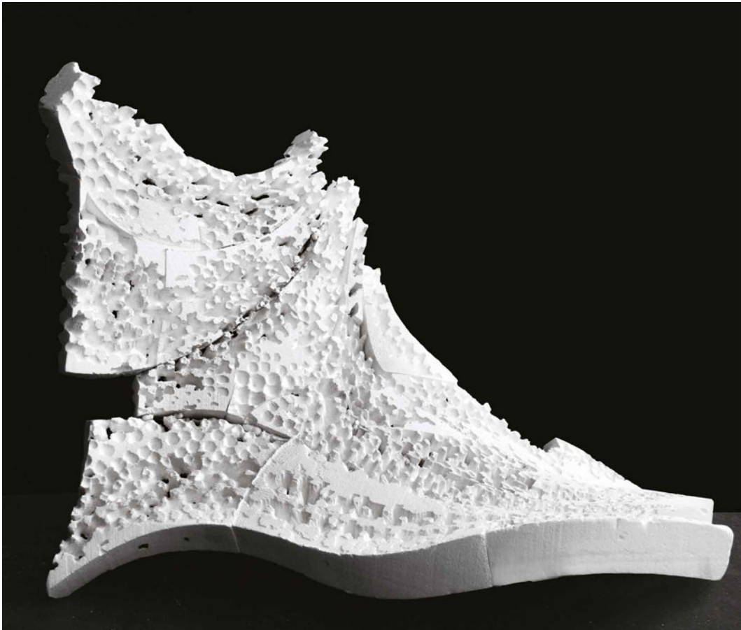
FIG. 4.2 Multi-mode Hybridity - volumetric cutting and milling are used together as a hybrid production strategy implementing two subtractive robotic fabrication methods.
