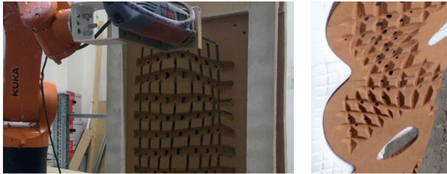
FIG. 2.19 Hybrid Assembly, The flexibility of the prototype is studied through prototyping in combination with the digital model that simulates the bending process of the 2D material into the desired 3D free form surface.
