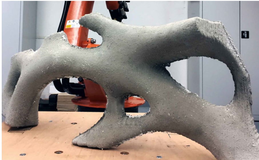
FIG. 4.15 Concrete branch prototype, with robotically produced formwork with two temporary mold parts.
