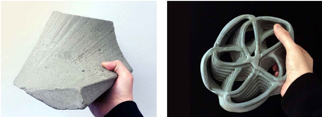
FIG. 2.3 Example of how the topology of fabrication affects the geometric qualities, Left: A cast concrete element with linear traces of Robotic Hot Wire Cutting tool on the surface; Right: Glazed Robotically 3D printed prototype with layered finishing surface quality.
