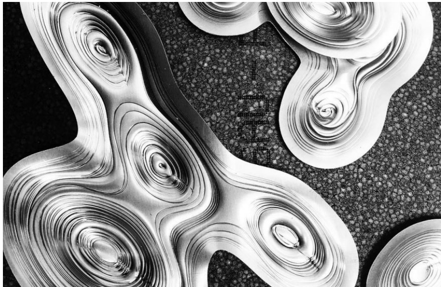
FIG. 2.17 Incremental Sheet Forming of 1mm thick aluminum to free-formed surfaces with embedded engravings to increase and control stiffness; Result of experiments in a design-to-production studio.
