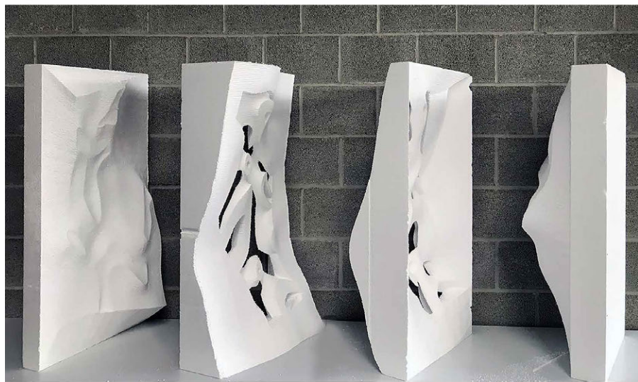
FIG. 4.18 The robotically produced four part mold of Hybrid Concrete prototype.
