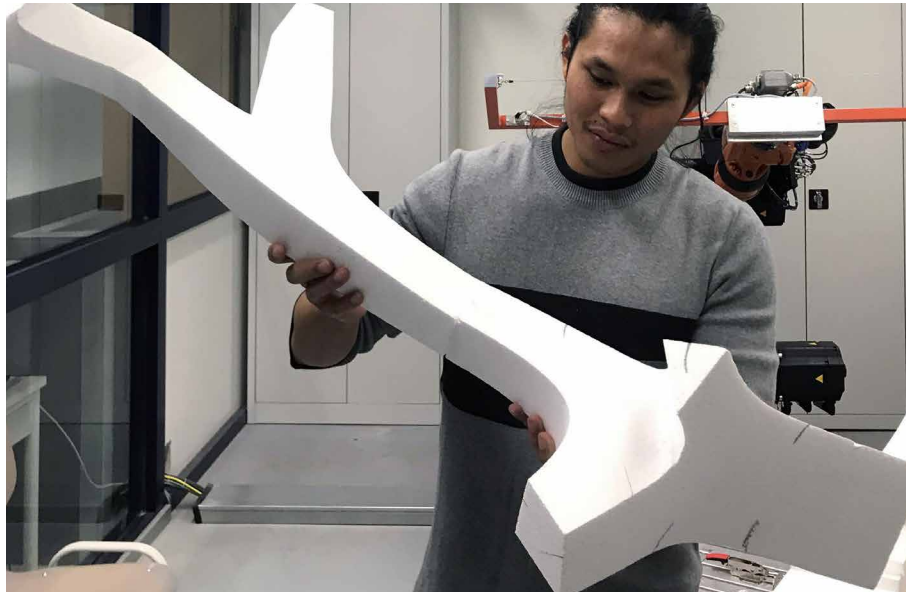
FIG. 2.5 Example of topology of fabrication and families of components: Robotically produced branching prototype with three and four branching node components.
