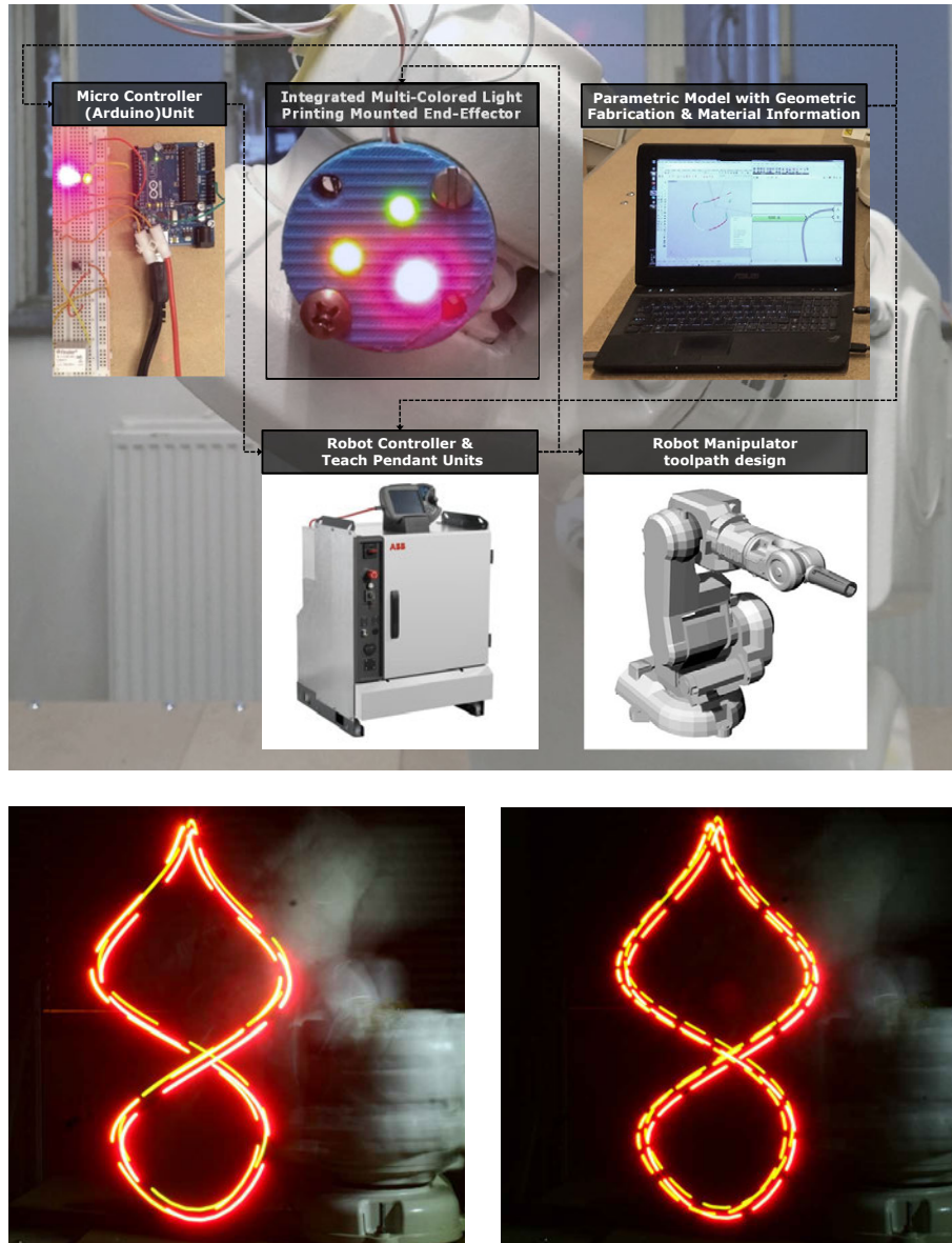
FIG. 2.9 Top: Establishing connections between the digital and the physical; Bottom: Robotic Light Printing with color changing and blinking pattern according to the digital model.
