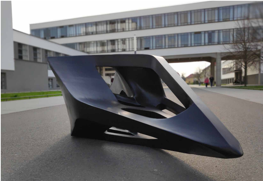
FIG. 4.6 Robotically Produced Fiber Glass Music Stage Table, Implementing Robotic Hot Wire Cutting combined with Robotic Milling where needed and as needed results in a smooth transition from curved to developable surfaces.
