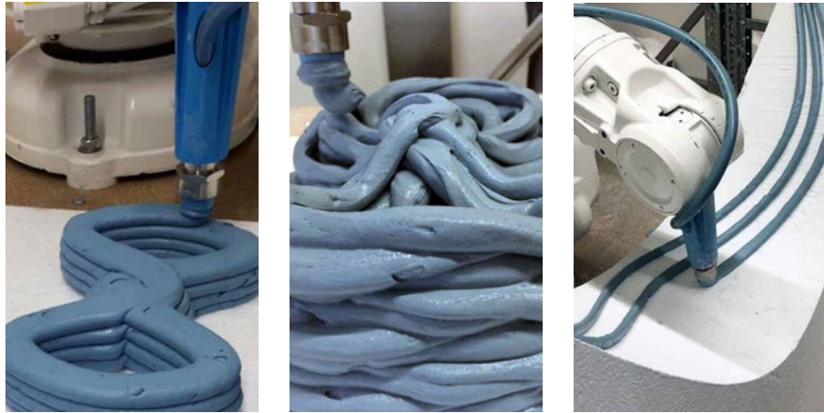
FIG. 2.13 Series of Robotic 3D Printing experiments studying different levels resolution for material deposition.
