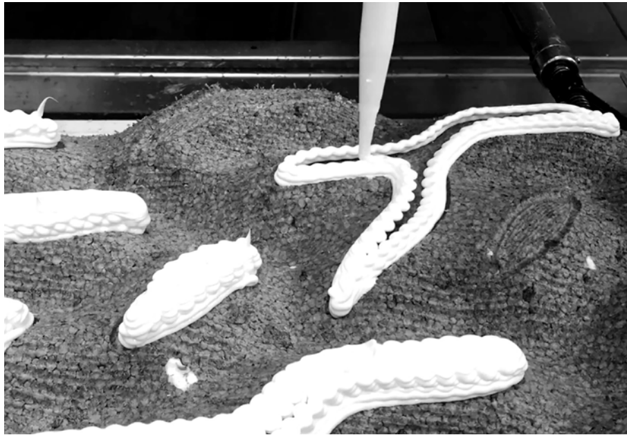
FIG. 4.25 Fortifying sine wave toolpath for silicone printing to increase the stability of printed material.
