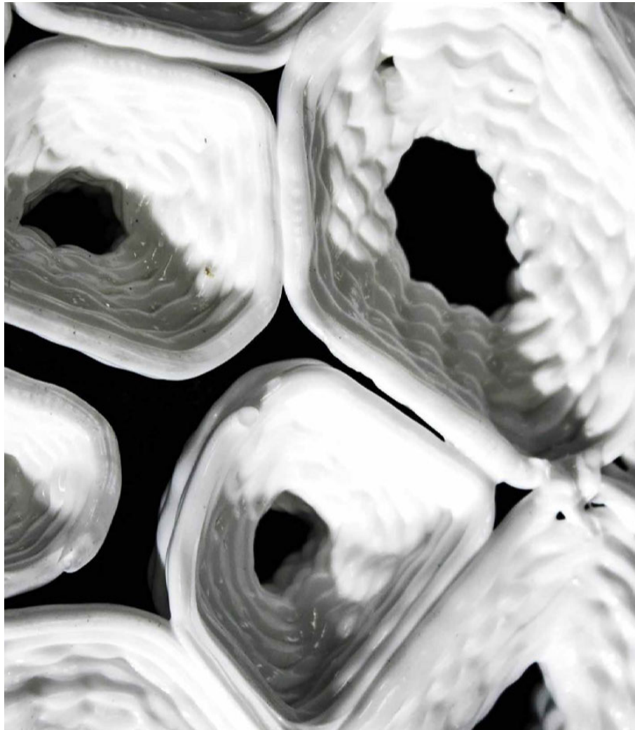
FIG. 4.34 Silicone cell on EPS surface, The fortifying sine wave smoothly disappear as the print reaches the tip of cantilever.
