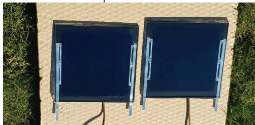
Figure 5(a) Estimated reflectance of the IR filter (b) A PV mini-module with and without implementation of the IR filter.
