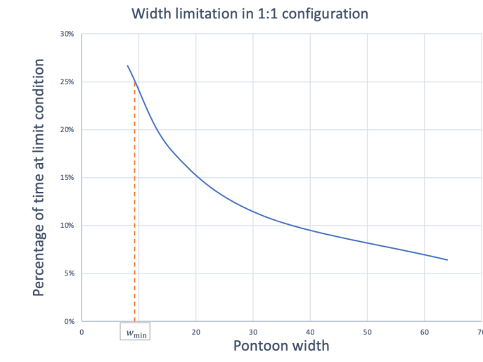
Figure 3.16: Time percentage of tilt and slant reaching 60^\circ as the pontoon's width varies.
