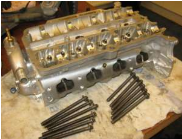
Figure 1.1. Cylinder head and the cylinder head bolts of an Opel Ampera. This vehicle was disassembled at Nedschroef Techno Centre in order to study the fasteners of a modern hybrid car. The cylinder head bolts have a length of 122 mm.
