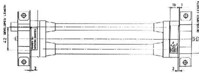
Fig-1.17 Mechanical drawing of the straight Ulysses nutation damper. The upper tube is the vapor tube whilst the lower one with the largest diameter is the liquid tube [courtesy Dutch Space].
