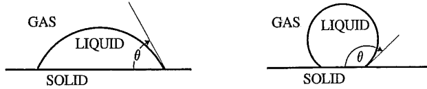
Fig-2.20 Wetting (left) and non-wetting conditions of a droplet on a plate [Schetz, 1999].
