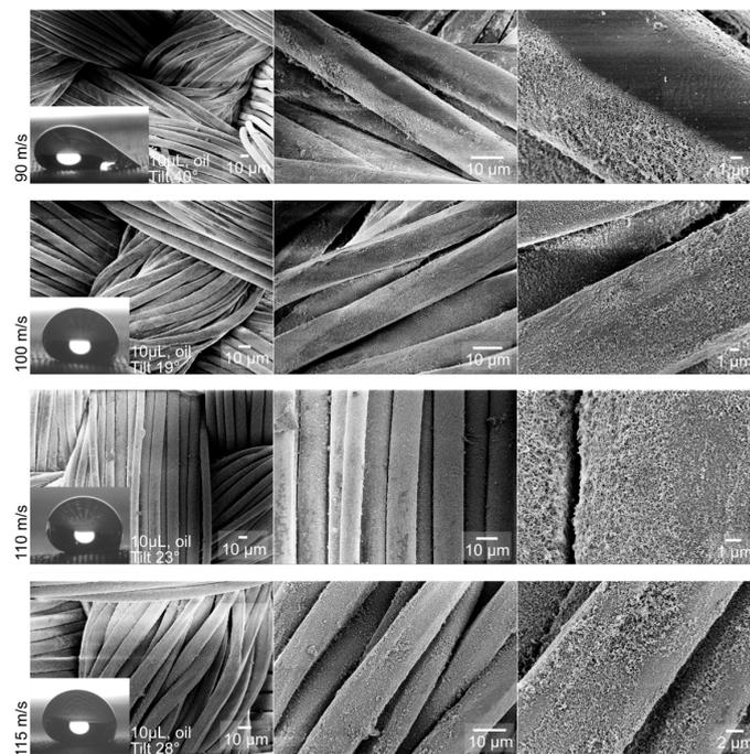
**Figure 7.** SEM images of superamphiphobic fabrics tested in a flat plate configuration at an angle of attack of  $20^\circ$  and in icing conditions. Each row consists of increasing magnification of a single fabric tested at the airspeed indicated on the left. The inset images are  $10\ \mu\text{L}$  oil droplets on the respective fabric sample following durability testing and tilted at the angle specified beside the image.
