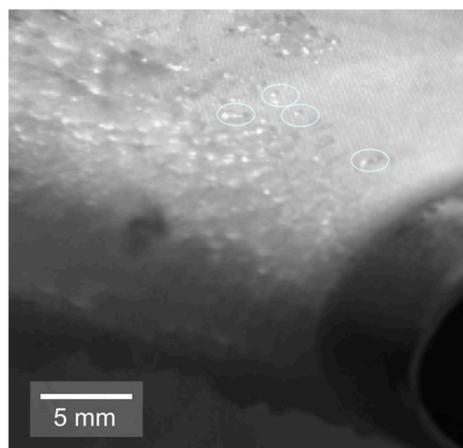
**Figure A3.** Ice formation on the fabric mounted on a NACA 0012 airfoil showing isolated feathery ice grains near the top side (circled) that become more dense and homogenous approaching the stagnation line.
