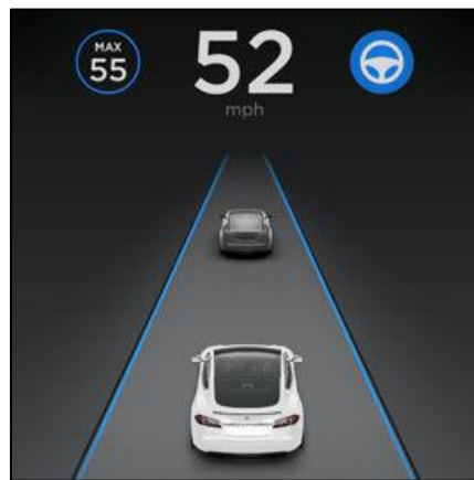
Figure 4. Conditions to initiate Autosteer
