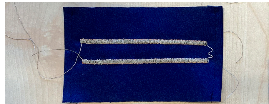
Figure 85. Optimised double row ZigZag sensor design
