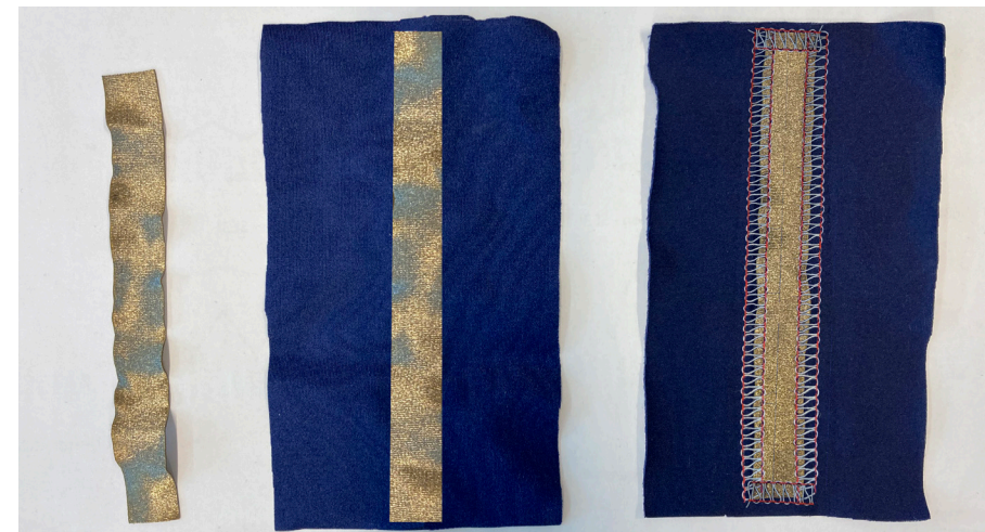
Figure 73. left to right: Conductive lycra strip and strip glued, strip stitched to 85% Ny substrate
