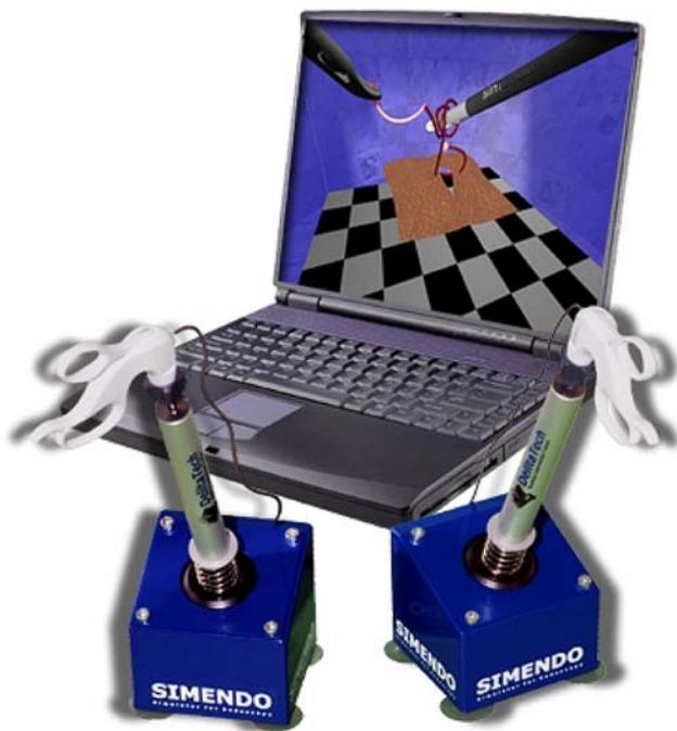
**Fig. 2** The SIMENDO, a virtual reality (VR) trainer produced by DelltaTech (courtesy of DelltaTech)
