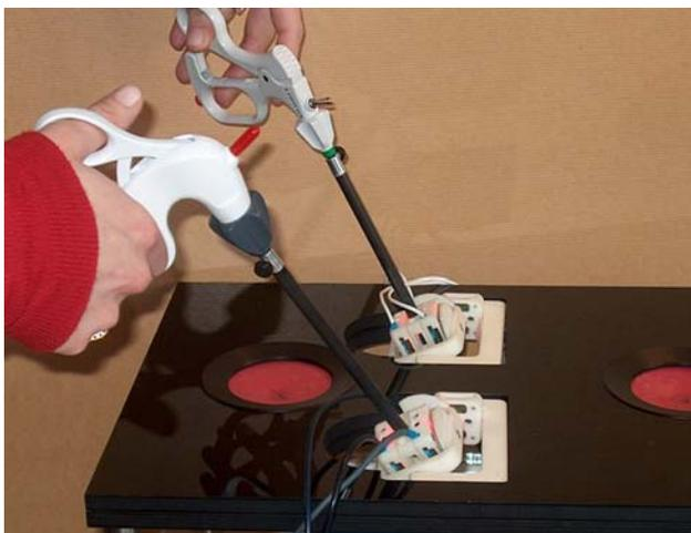
**Fig. 3** The TrEndo tracking system designed to measure movements of laparoscopic instruments in training setups
