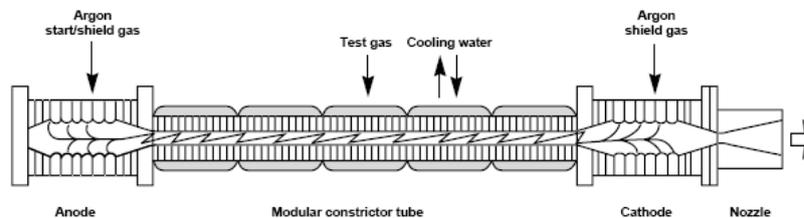
Figure 1: Schematic drawing of the segmented arc-heater
