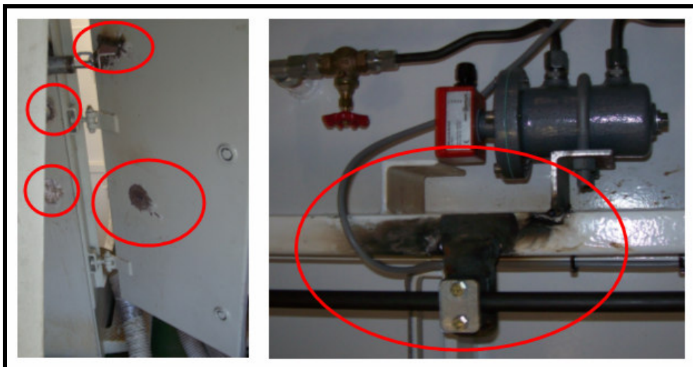
Figure 1 Damage to paint work due to welding at IHC Beaver Dredgers
