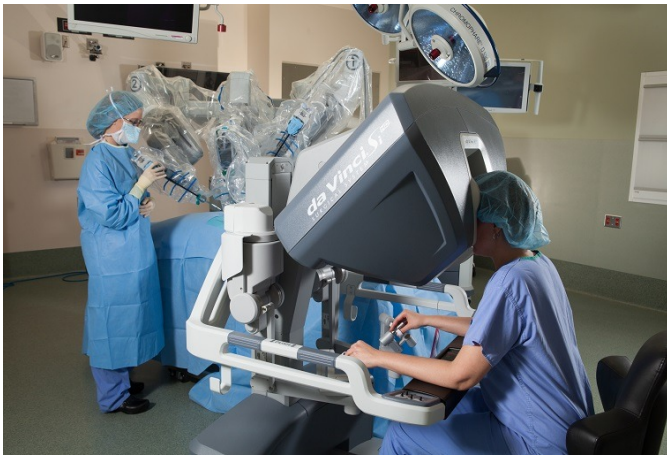
Figure 1: Da Vinci Si system, with on the left the surgery robot above a patient and on the right the master interface where the surgeon is seated, controlling the robot.
