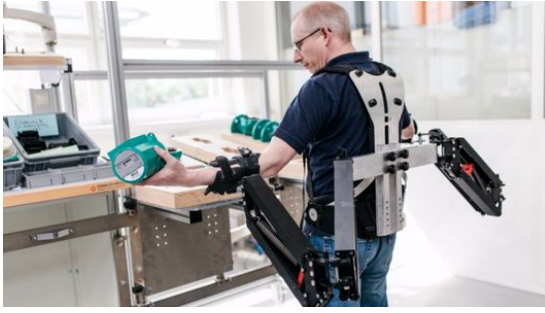
Figure 11: 'Robo-Mate', an exoskeleton arm support using two linked 4-bar mechanisms [5]
