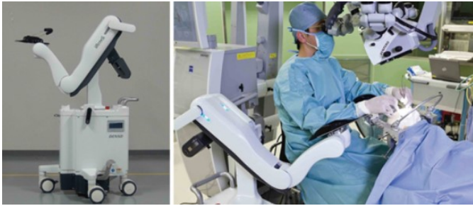
Figure 18: iArmS arm support system designed for multiple types of surgery, can be used in a seated as well as a standing posture. The picture on the right shows microscopic neurosurgery with the iArmS, reducing fatigue and increasing stability of the surgeon's hand.
