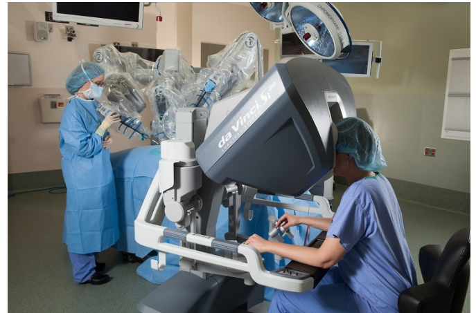
Figure 1: Da Vinci Si system, with on the left the surgery robot above a patient and on the right the master interface where the surgeon is seated and controlling the robot.
