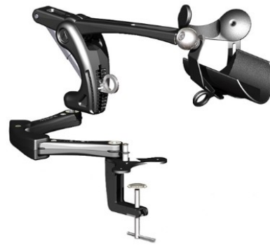
Figure 15: 'Armon Edero', a single lever arm support actuated by an adjustable extension spring [8].
