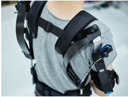
Figure 17: 'Skelex-360', an exosuit with bending beams acting as actuators and structural components. [11].
