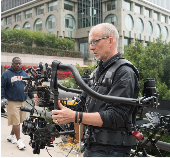
Figure 26: Exhauss exoskeleton for the stable carry of heavy gimbal videocamera systems
