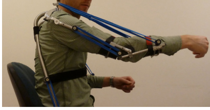
Figure 16: 'A-gear', a double-lever arm support mechanism supporting the arm in two places [10].
