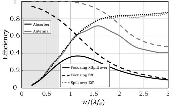
Fig. 9. Focusing and spill-over efficiencies for both ideal antenna and absorbers, with a square dimension of side length  $w$ , under a reflector with  $f_{\#} = 2$ . The grey area indicates the region where the product of the two efficiencies, for the absorber and antenna feeds, are comparable.
