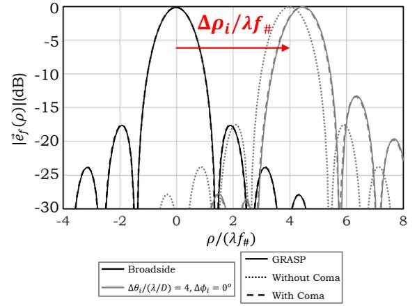
Fig. 6. Direct fields focalized by a reflector with  $f_{\#} = 0.6$  and  $D = 100\lambda$ . The reflector is illuminated by two plane waves: at broadside and with  $\Delta\theta_i/(\lambda/D) = 4$ ,  $\Delta\phi_i = 0^\circ$ . Dash and dotted lines represent the fields with and without including the coma phase term in the PWS, respectively. The solid lines are relevant to the fields calculated with GRASP.
