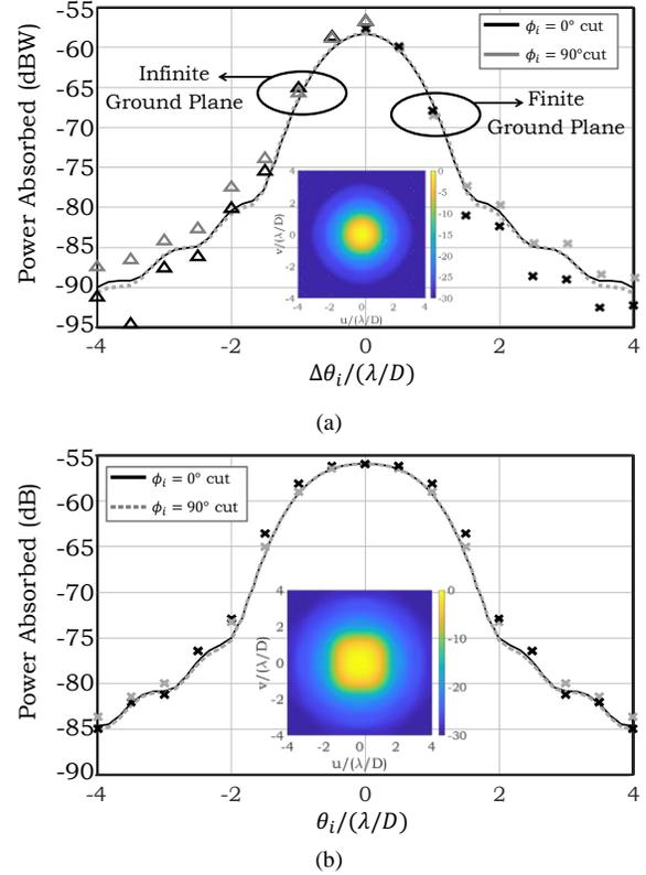
Fig. 13. Power absorbed versus the plane wave incident angle (non-normalized angular response) of a linear strip absorber with side length  $w$  coupled to a reflector with  $f_{\#} = 0.6$ : (a)  $w = \lambda f_{\#}$  and (b)  $w = 2\lambda f_{\#}$ . Solid lines: calculated by using (14). Marks: obtained via full wave simulations. The inset illustrates the 2D response in  $u$ - $v$  coordinates
