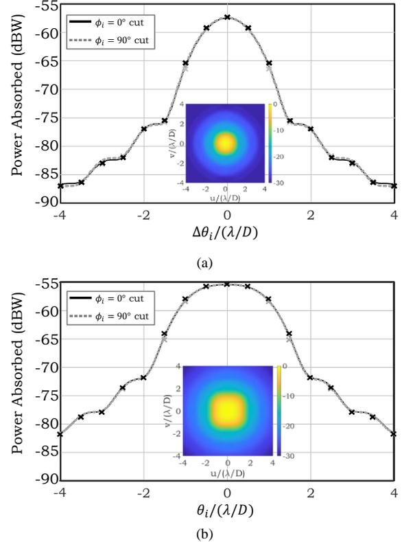
Fig. 11. Power absorbed versus the plane wave incident angle (non-normalized angular response) of a linear strip absorber with side length  $w$  coupled to a reflector with  $f_{\#} = 2$ : (a)  $w = \lambda f_{\#}$  and (b)  $w = 2\lambda f_{\#}$ . Solid lines: calculated by using (18). Cross marks: obtained via full wave simulations. The inset illustrates the 2D response in  $u$ - $v$  coordinates
