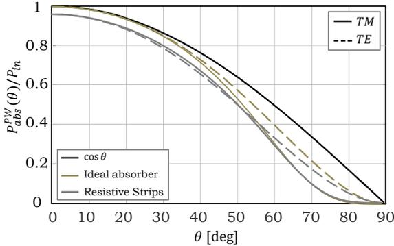
Fig. 2. Power absorbed by an ideal planar absorber and a strip absorber for a  $\hat{\theta}$ - (TM) and  $\hat{\phi}$ -polarized (TE) plane wave incidence at different incidence angles. Both designs use back shorts at  $\lambda/4$  distance. The curves are normalized to  $P_{in} = S_i A$ .
