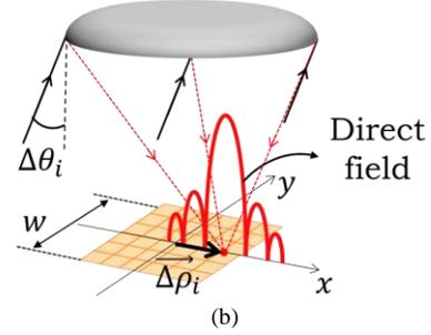
Fig. 8. (a) Angular response to a plane wave impinging from  $\Delta\theta_i$  of both an ideal absorber, and a uniform aperture antenna coupled to a parabolic reflector with  $f_{\#} = 2$ . The different curves correspond to several absorber and antenna sizes. (b) Sketch showing the detecting device (antenna/absorber) and direct field for a case of a squinted plane wave incidence.
