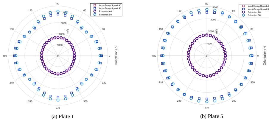
Figure 4.7: Group speed extraction of simulated signals
