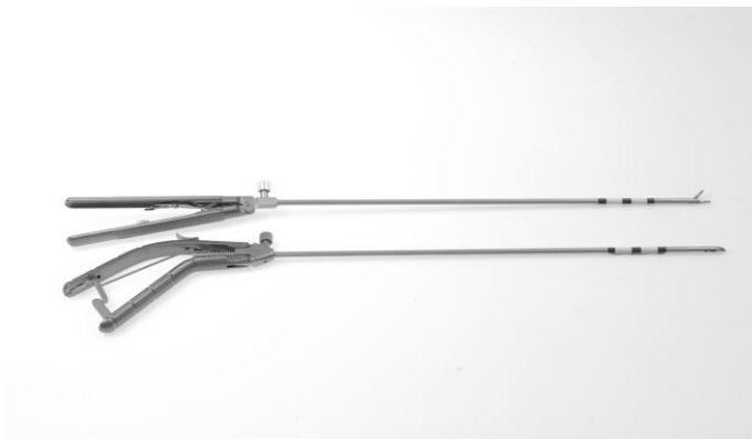
Figure 2. The needle holders (Karl Storz, Tutlingen, Germany) are marked with the black-yellow tags on the shaft to enable video tracking.
