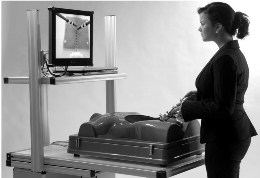
Figure 1: ProMIS Augmented Reality Laparoscopic simulator (Haptica, Dublin, Ireland), with needle-holders (Karl Storz, Tutlingen, Germany) and versaport trocars 5mm (Tyco Auto Suture, New Haven, USA)
