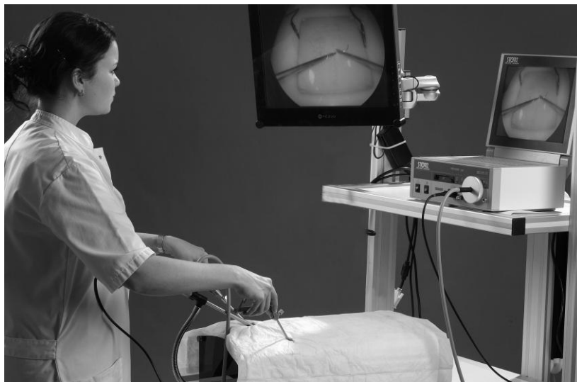
Figure 1: Traditional box trainer, containing a foam suturing pad (Limbs & Things Limited, Bristol, United Kingdom), a Telepac system with endoscope (Karl-Storz Endoscope, Tuttlingen, Germany), video monitor (Neovo X17a) and needle holders (Karl-Storz Tuttlingen, Germany).
