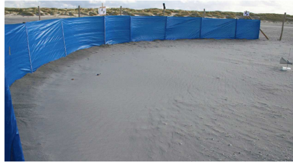
Figure 2: Sand screen, checkerboard targets and saltiphone; Accumulation of sand in front of the screen is visible as well.
