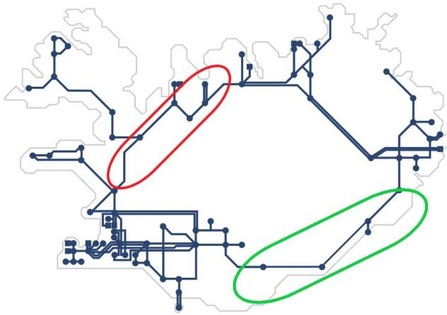
**FIGURE 8.** Icelandic power system, the corresponding corridors of lines connecting two parts of the network are outlined in red and green for the northern and southern ring connections respectively. [37].
