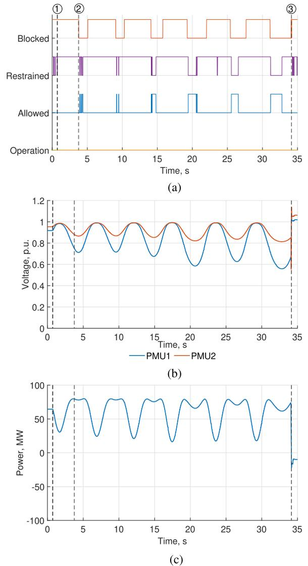
**FIGURE 17.** Protection algorithm response to Event 3 data. The dashed line marked as ① shows the start of the OOS event at 0.5 seconds. (a) the protection algorithm signals from the controller, (b) the voltage at the two measurement locations in the southern corridor and (c) the measured power in the southern corridor during the event.
