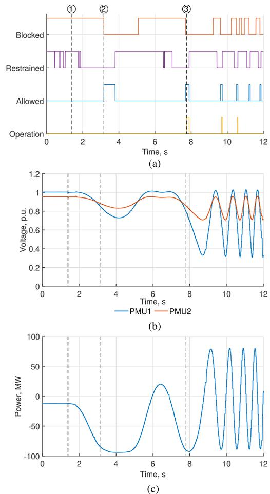
**FIGURE 15.** Protection algorithm response to Event 1 data. The dashed line marked as ① shows the start of the OOS event at 1.3 seconds. (a) the protection algorithm signals from the controller, (b) the voltage at the two measurement locations in the southern corridor and (c) the measured power in the southern corridor during the event.
