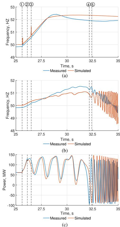
**FIGURE 10.** OOS event 2 measured and simulation values. (a) the frequency in the south-west center of inertia, (b) the frequency of the east center of inertia and (c) the active power flow in the southern corridor, where the OOS event takes place. ① - the start of the event with the loss of load, ② - inter trip on the 220 kV substation at the southern corridor, ③ - north corridor disconnection from overload, ④ - first pole slip in measured values, ⑤ - first pole slip in simulation.
