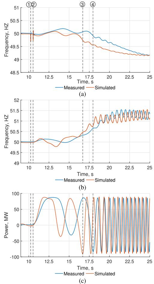
**FIGURE 9.** OOS event 1 measured and simulation values. (a) the frequency in the south-west center of inertia, (b) the frequency of the east center of inertia and (c) the active power flow in the southern ring connection, where the OOS event takes place. ① - the start of the event with the fault in the north corridor substation, ② - fault clearance, ③ - first pole slip in simulated values, ④ - first pole slip in measured values.
