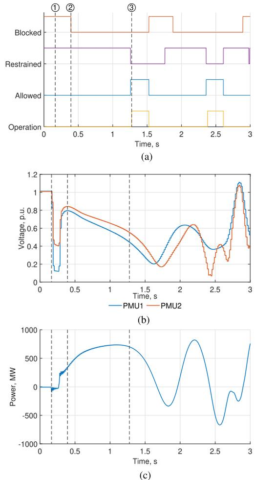
**FIGURE 7.** Protection algorithm response signals, voltages at both ends of the transmission line and active power through the line during an unstable power swing and subsequent OOS condition. (a) protection algorithm signals in the external controller, (b) the voltage magnitudes at both ends of the protected transmission line and (c) the active power through the protected line.
