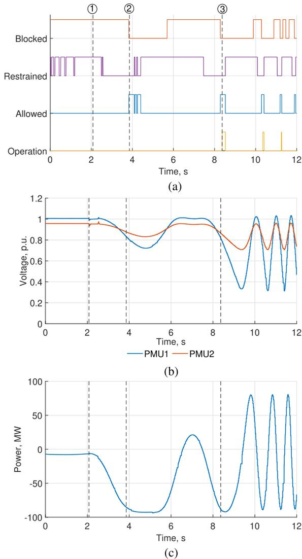
**FIGURE 16.** Protection algorithm response to Event 2 data. The dashed line marked as ① shows the start of the OOS event at 2.1 seconds. (a) the protection algorithm signals from the controller, (b) the voltage at the two measurement locations in the southern corridor and (c) the measured power in the southern corridor during the event.
