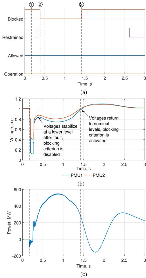
**FIGURE 6.** Protection algorithm response signals, voltages at both ends of the transmission line and active power through the line during a stable power swing in the network. (a) protection algorithm signals in the external controller, (b) the voltage magnitudes at both ends of the protected transmission line and (c) the active power through the protected line.
