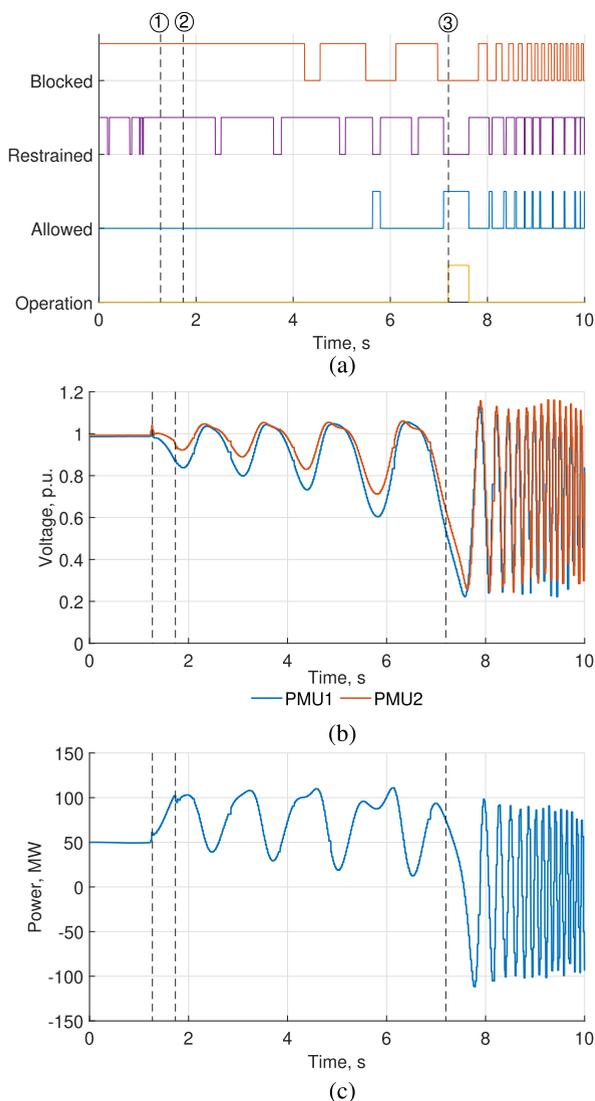
**FIGURE 18.** Protection algorithm response to Event 2 data. The dashed line marked as ① shows the start of the OOS event at 1.3 seconds. (a) the protection algorithm signals from the controller, (b) the voltage at the two measurement locations in the southern corridor and (c) the measured power in the southern corridor during the event.
