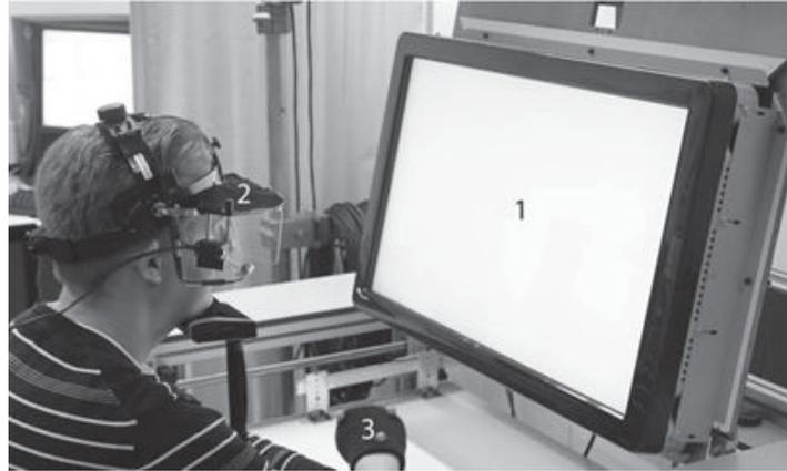
**Figure 4-1:** The setup at the EMC used for measuring loss of eye-hand coordination and cognitive skills. (1) touch screen, (2) infrared eye-tracking system, (3) infrared motion detection system [31]
