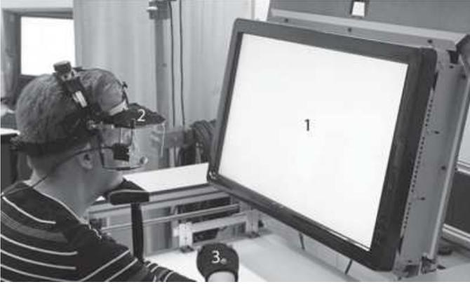
Fig. 3. The setup at the EMC used for measuring loss of eye-hand coordination and cognitive skills. (1) touch screen, (2) infrared eye-tracking system, (3) infrared motion detection system [40]
