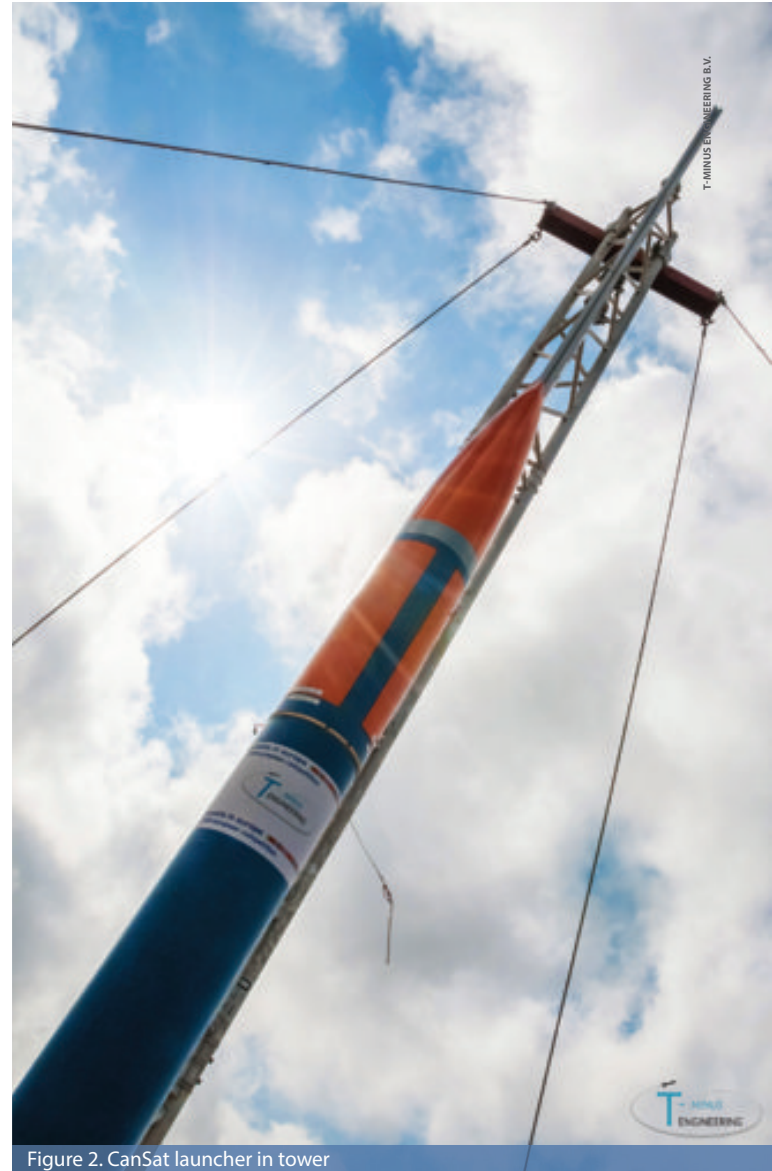
Figure 2. CanSat launcher in tower
