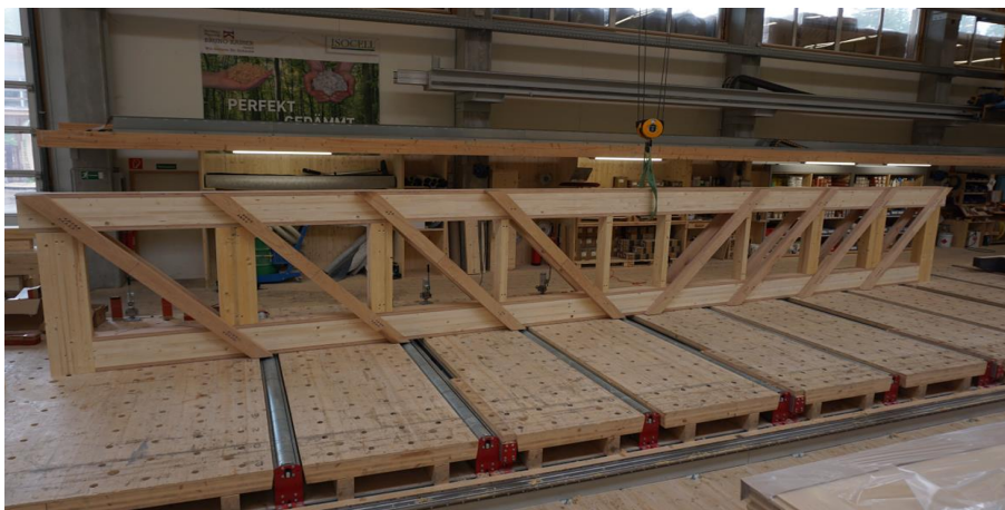
Figure 1.1: FaNaBu truss concept with composite upper and lower chords and LVL tensile diagonals connected using inclined screws [25, p. 63].
