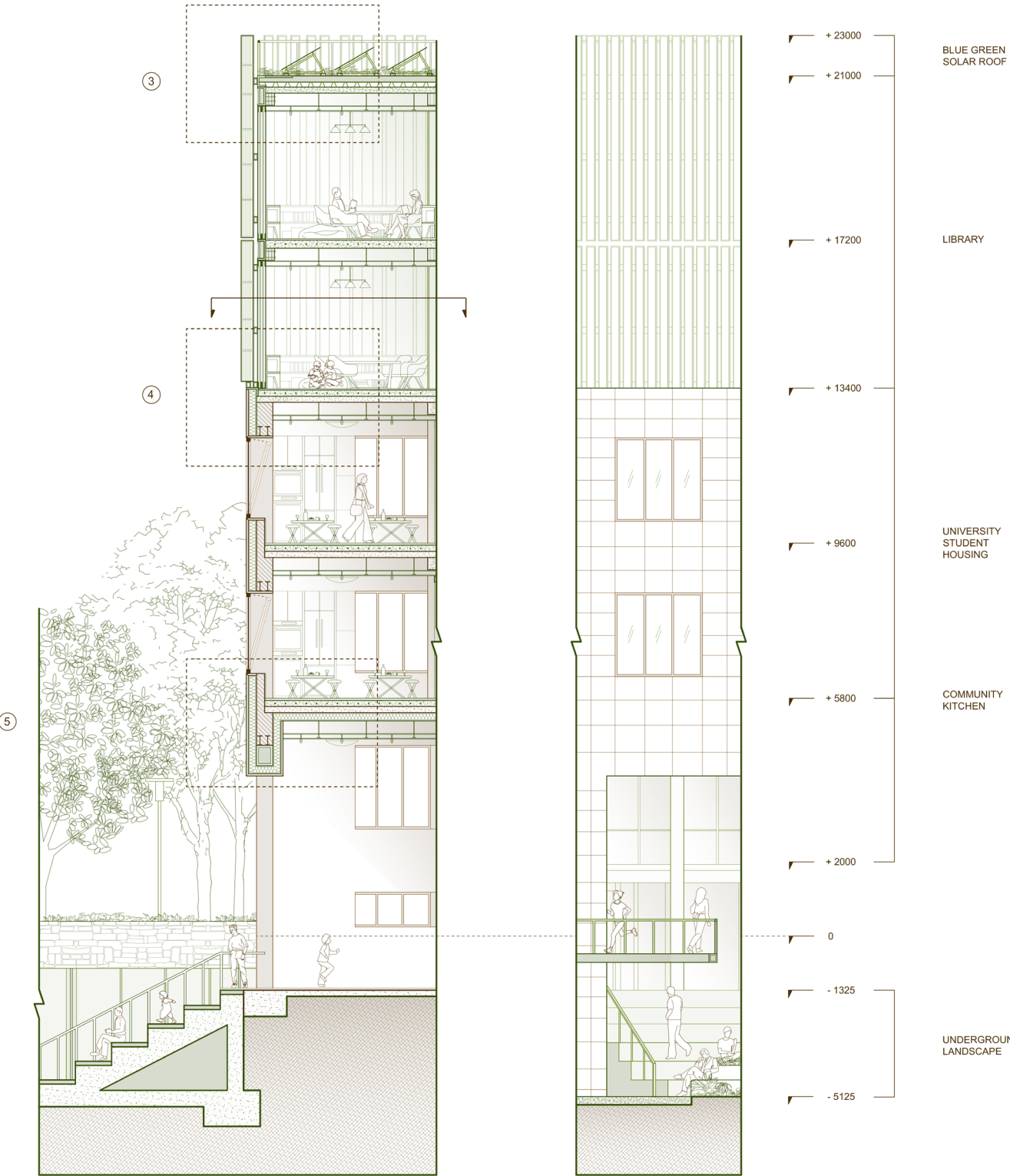
TRANSFORMED FACADE FRAGMENT PLAN, SECTION, ELEVATION AND DETAILS
