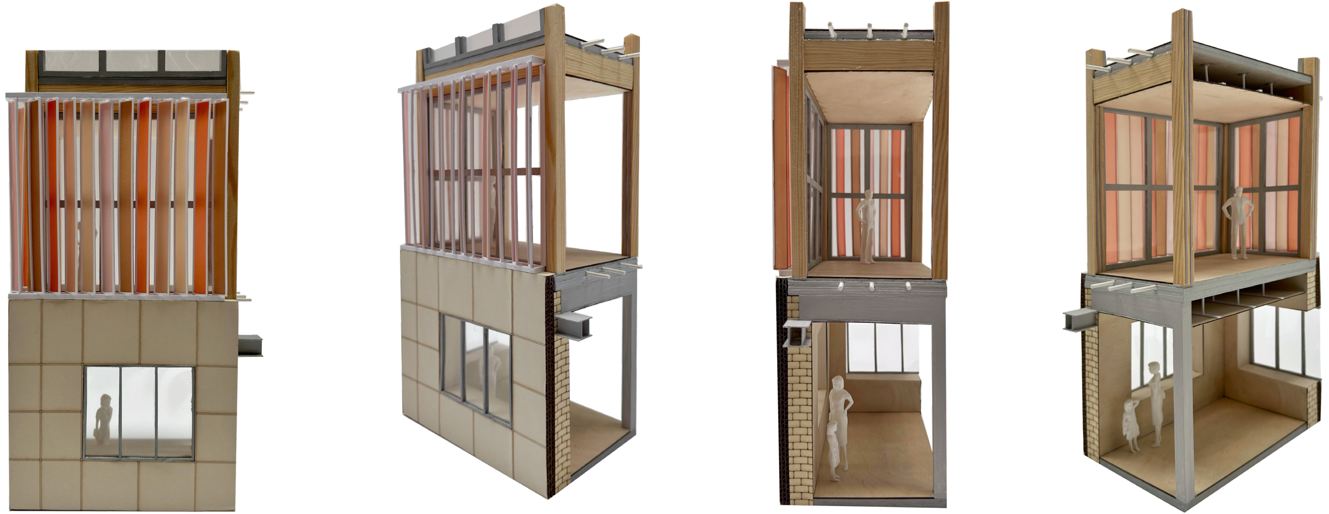
P5 | 1:25 | Facade Fragment Physical Model
