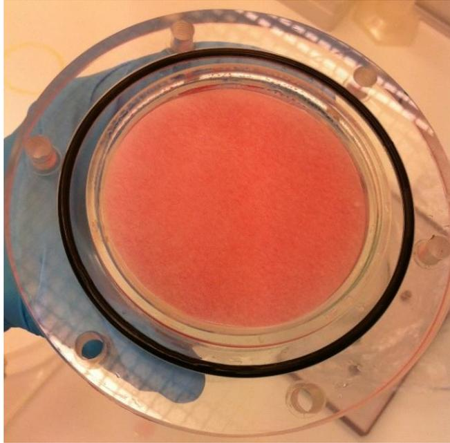
Figure 5.5.3: Collagen gel concentration method. All the equipment has been turned upside down; the nylon mesh layer and the filter paper have been applied atop of the gel prior to the attachment of the porous plate and part C. The plug stays in place (due to large friction forces) when the apparatus is turned upside down. Gel was separated from the edges of the acrylic tube by using a scalpel.
