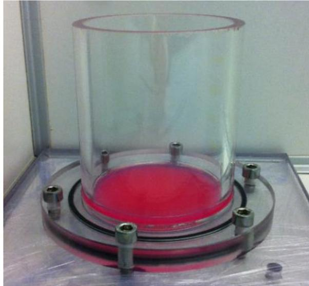
Figure 5.5.1: Apparatus used for collagen solution casting (part A and B).
