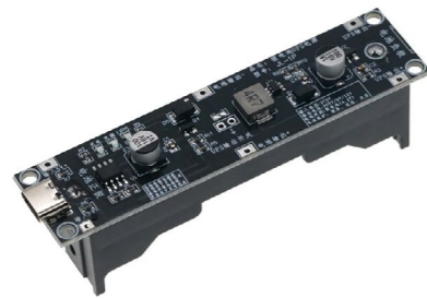
Figure 7.8: Otronic 18650 battery holder with an integrated charger and a 5 V step-up module (USB-C) https://www.otronic.nl/18650-batterijhouder-met-lader-en-5v-step-up-modul.html
