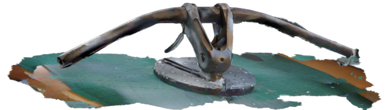
Figure 8.1: 3D scan of a handlebar in Crealtyscan application (before cleaning up the mesh)
