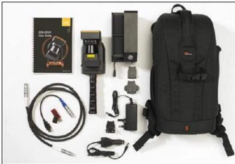
Figure 5- Mobile LiDAR device used for the cave scanning (ZEB-REVO GeoSLAM).
