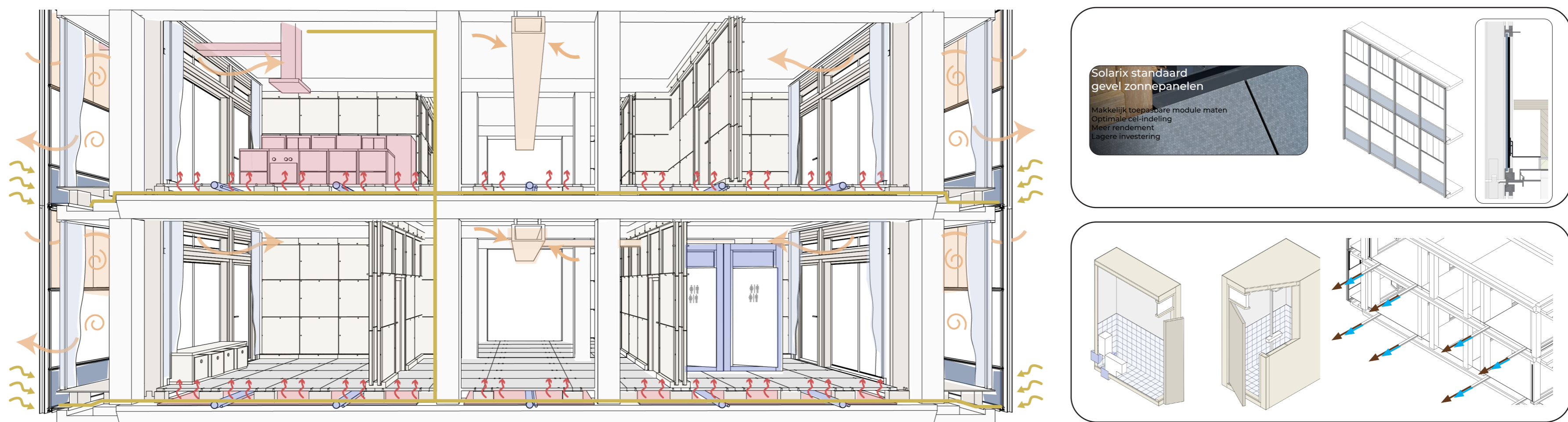
Climate design | Future proof EWI high-rise section with sustainable energy and heating systems with adaptable water and sewage system
