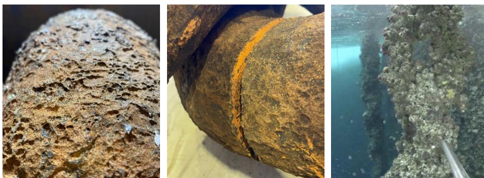
Figure 1.3. Corrosion pits (left) and fatigue crack (centre) in used mooring chain links, and marine growth deposits on submerged mooring chains (right) [7].
