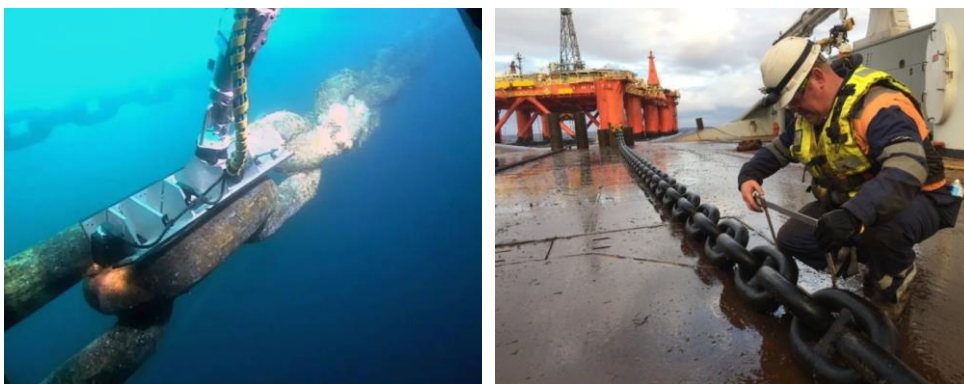
Figure 1.6. Examples of visual inspection of mooring chains in wet (left) and dry (right) conditions [20-21].
