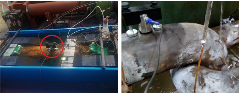
Figure 1.10. Sample illustration of AE testing of mooring chain links [58-59].
