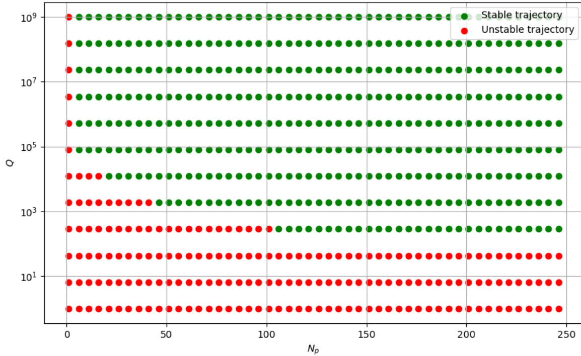
Figure 4.8: Closed-loop stability map for varying control parameters Q and prediction horizon N_p , control horizon N_c taken equal to 1.
