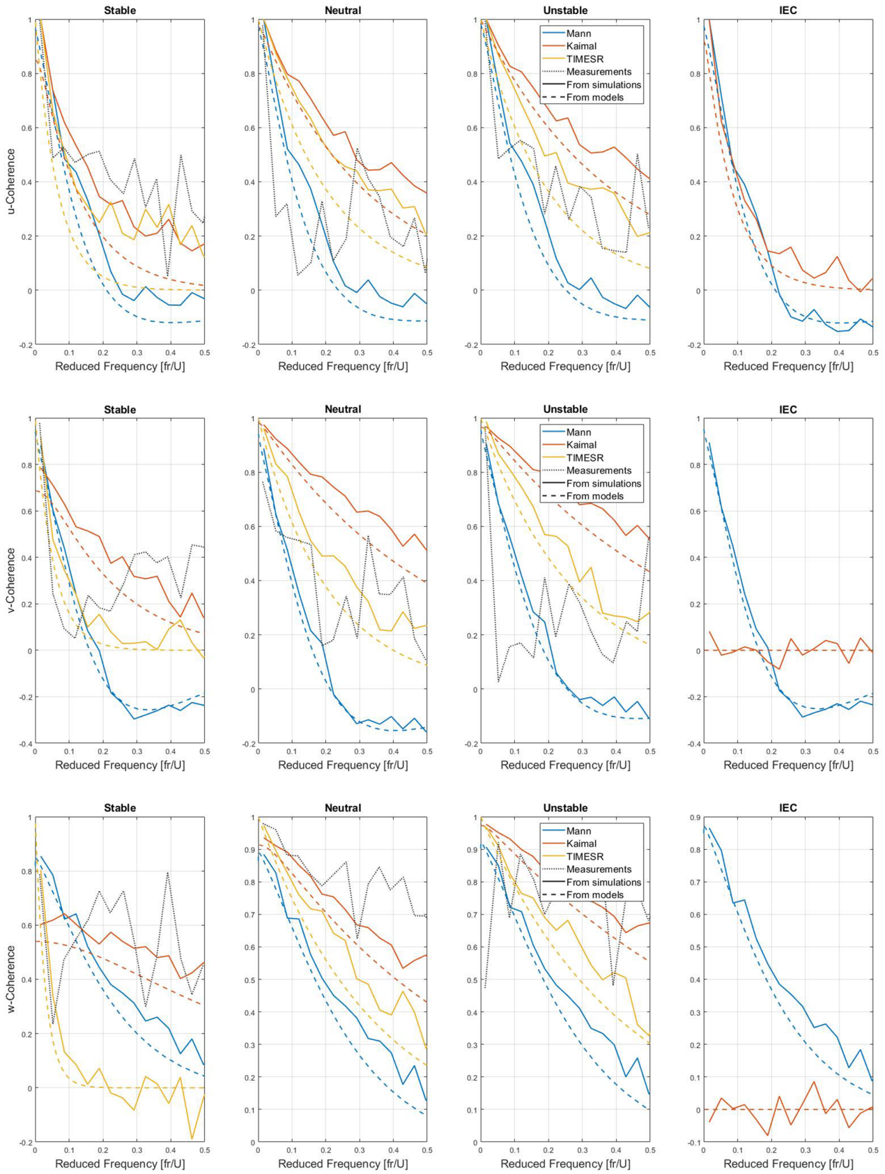
Figure C.1: Coherence in three directions between hub height and 20 meters below the hub at 7.5 m/s as a function of reduced frequency
