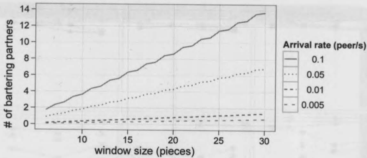
Figure 3.5: Expected number of bartering partners for the window-based piece selection policy with different window size and peer arrival rate. The parameters are taken from Table 3.1.
