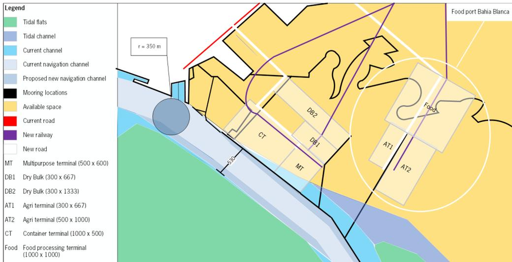
Figure 12.1. Conceptual design of the optimisation.
