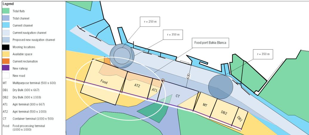
Figure 12.2. Conceptual design of the South expansion.
