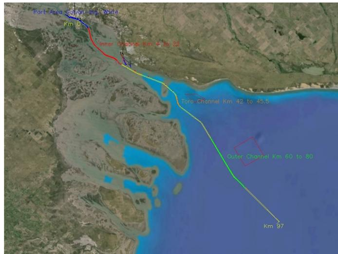
Figure B.1. The access channel and the dredged stretches.
