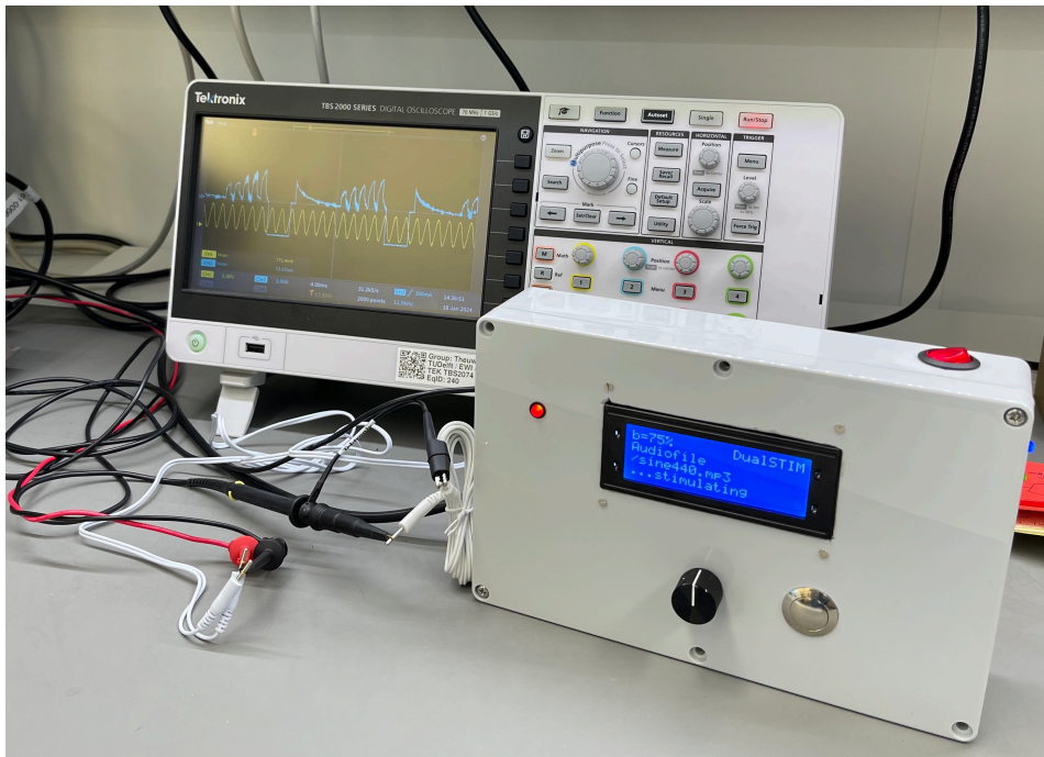
Figure 5.1: Distorted burst: Electrical stimulation [mA] in blue, acoustical stimulation [V] in yellow.
