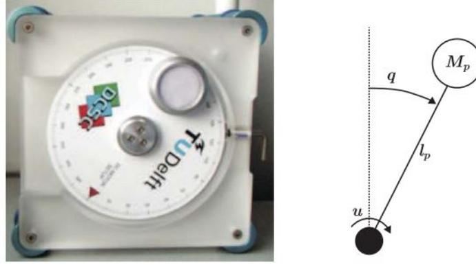
Figure 2-1: Inverted Pendulum [1]
