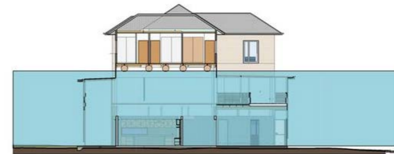
Figure 81. Cross Section showing how the Queenslander house floats using the pontoons (JDA, 2011)
