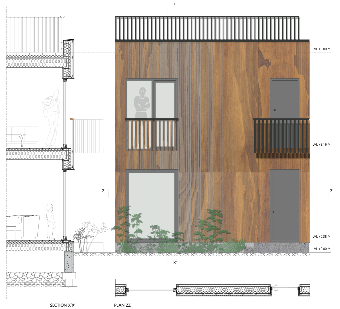
Figure 176. Difference in Wall section and Elevation of Dry and Flooding Houses (Authors own diagram)
