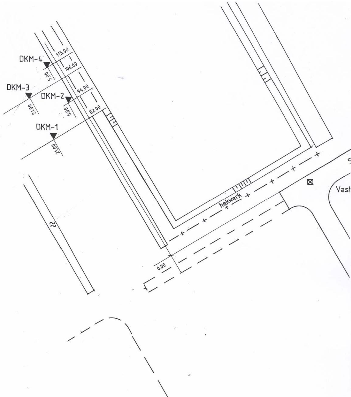
The positions of the first four CPT's on the test site at the Schuttevaerstraat in Wolvega
