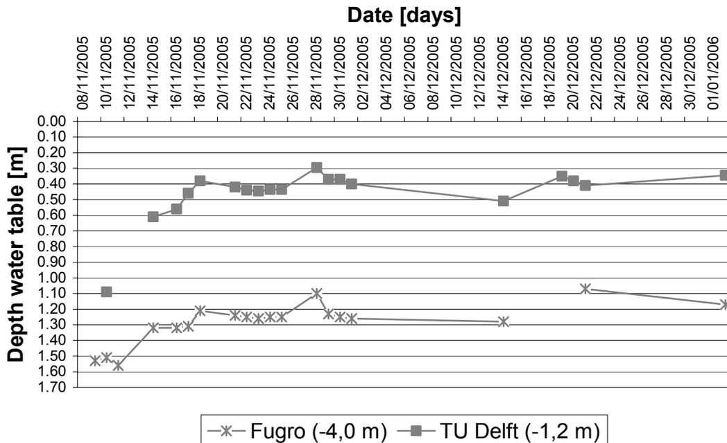
Figure 22 Depth of water table of the observation wells
