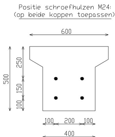
Figure 8 Front view of the foundation strip
