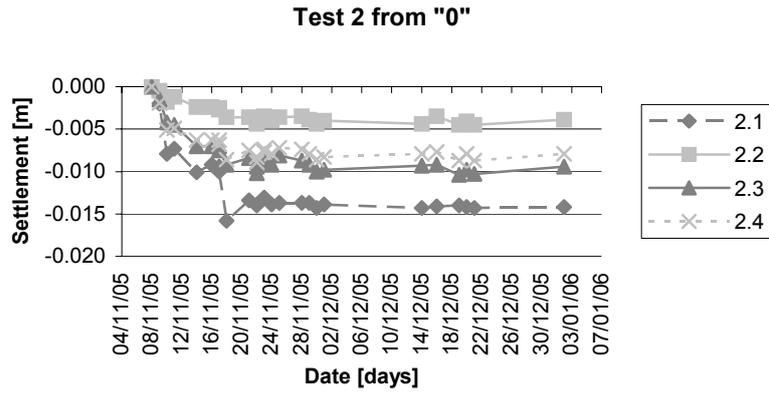
Figure 26 Settlement of the Reference Test Facility as plotted from the origin
