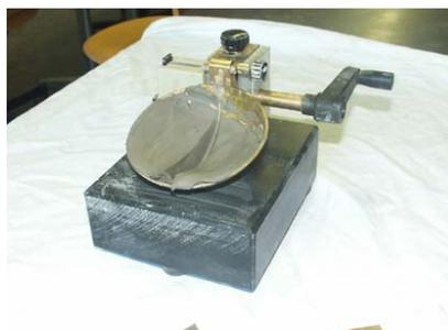
Figure 7 Casagrande device
