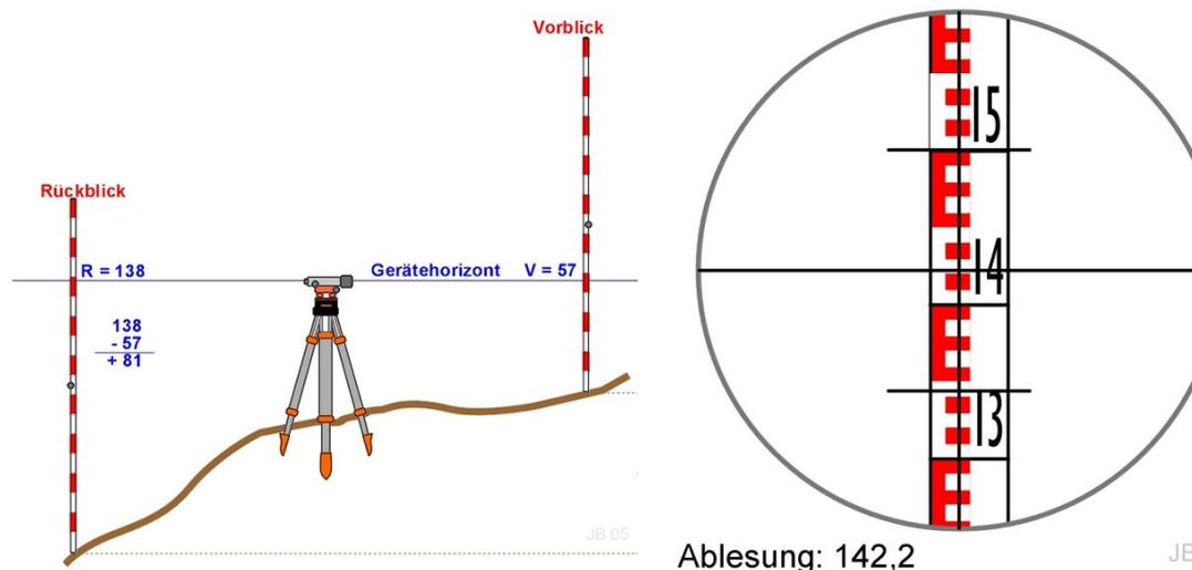
Figure 13 Levelling Measurement Equipment
