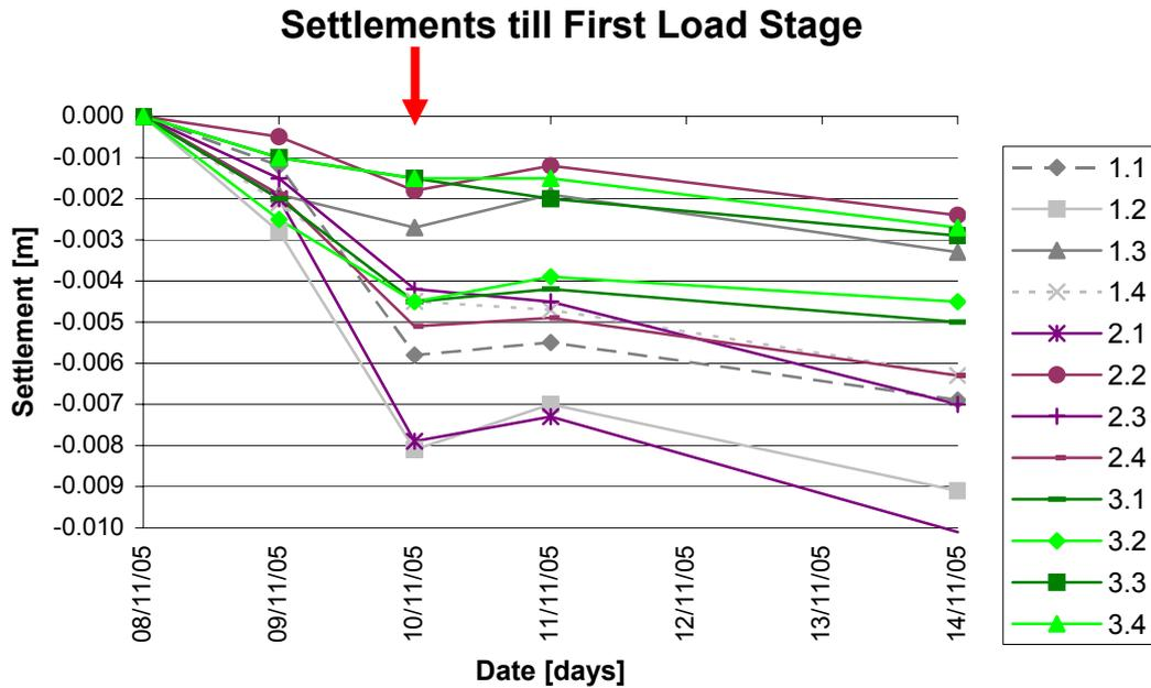
Figure 15 Settlements till the First injection; the red arrow marks the day of the first load stage
