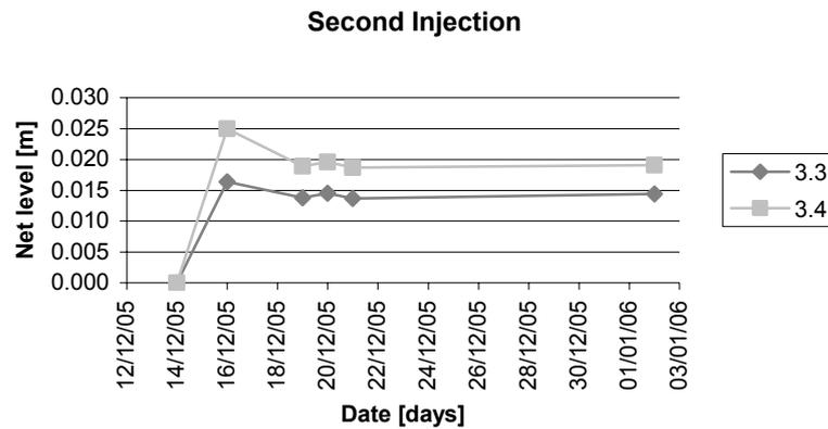
Figure 18 Lift of the second injection
