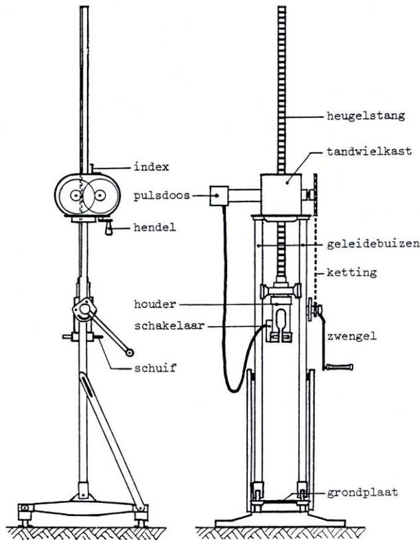
Total overview of the hand sounding construction. On the test site in Wolvega were the steel profiles [L] absent. In stead of the steel profiles there were ground anchors and the second time there was a crane who delivered the contra weight.
