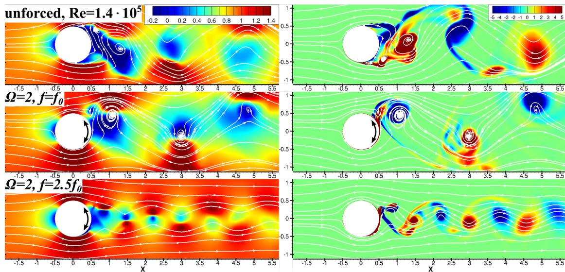
**Figure 4.** Axial velocity (left) and  $z$ -vorticity (right) for simulations with various  $\Omega$  and  $f$ .
