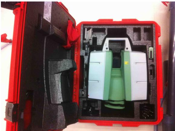
Red trunk with Leica C10 scanner
