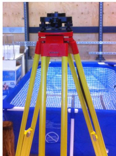
**step 3 level tripod with tribrach**
