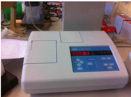
Figure 4.5: Hach 2100N Turbidimeter
