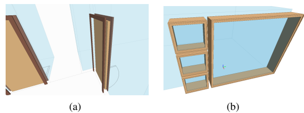
Figure 8: Example of IfcDoors and IfcWindows .
