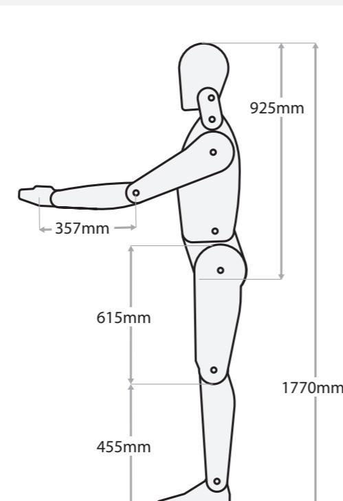
Figure 10. DINED measurements of European adult males applied to a 2D mannequin. Adapted from Link, 2016.
