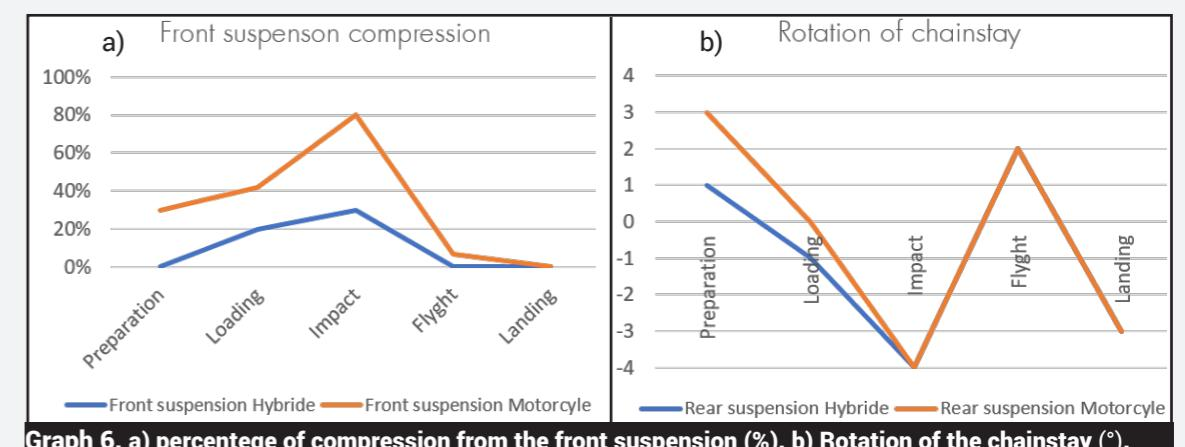
Graph 6. a) percentage of compression from the front suspension (%). b) Rotation of the chainstay (°).
