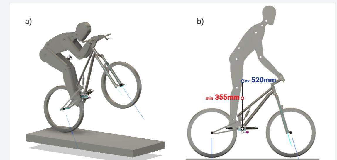
Figure 11. a) Mannequin in 3D used to locate the center of gravity. b) Average and minimum height of the center of gravity. Adapted from Link, 2016.
