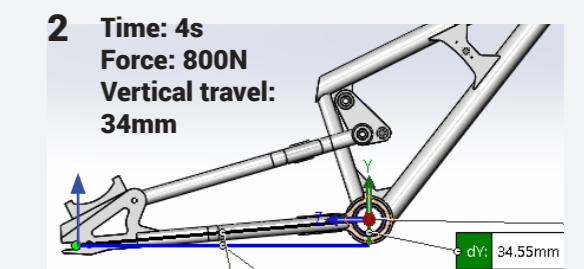
The rider climbed over the bicycle and is in a static position (sag position).
