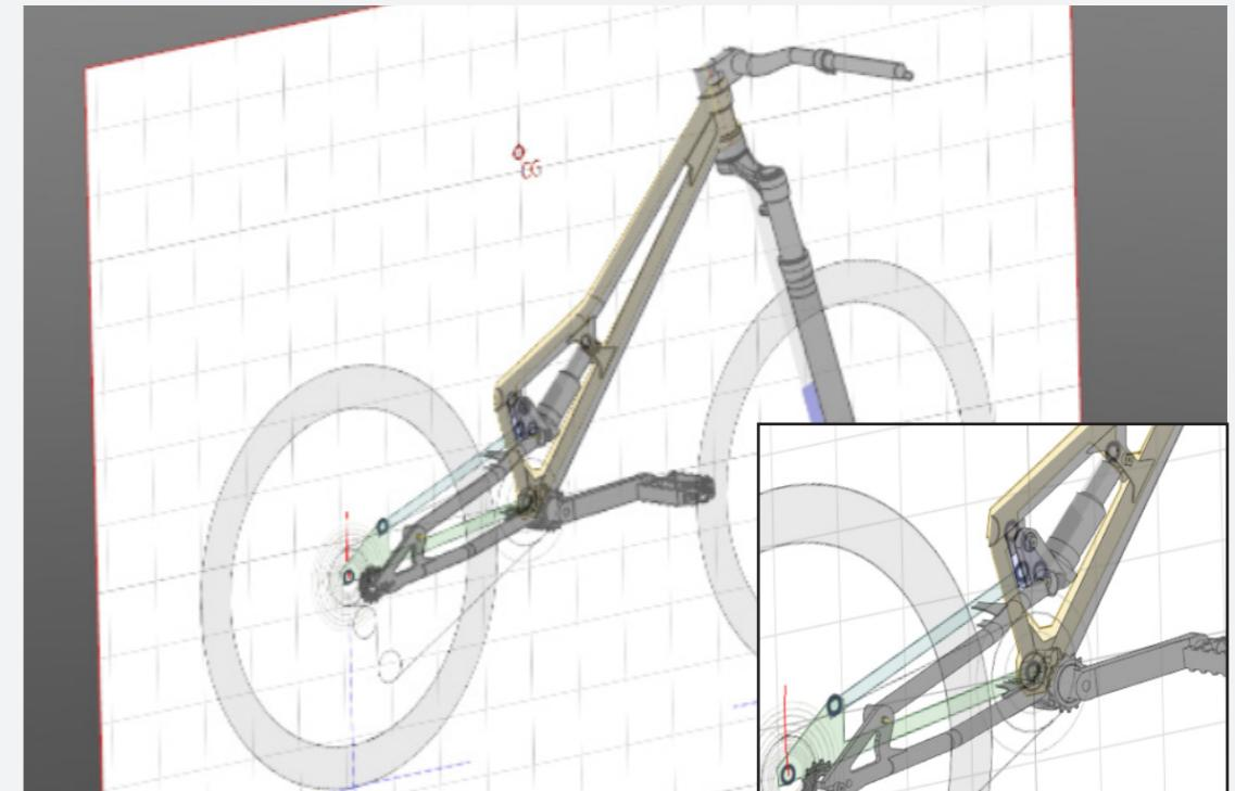
The main components of the frame were assembled together with the use of articulated unions, most of the time pin revolute unions (it restricts 5 degrees of freedom and lets free one degree of rotation). With the use of this unions it could be directly observed whether there would be any collision of components along the whole distance traveled by the suspension.
