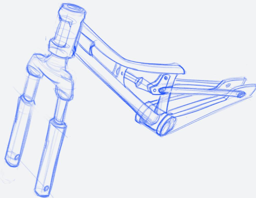
Parametric 3D drawing software has been used to give shape to the full complexity of the design. Once the design was completed, drawings and other files have been facilitated to a metal manufacturer specialized in building motorcycle frames (Derivados Del Motor S.L.) who have built the final model.
