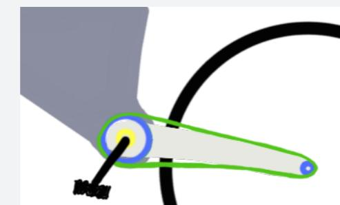
Figure 36. Bottom bracket pivot
