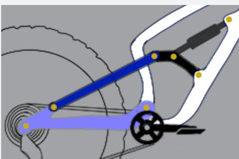
Figure 33. Single pivot linkage
