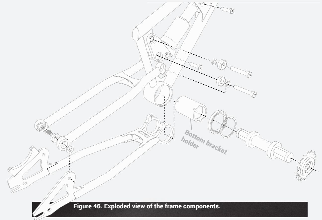
Figure 46. Exploded view of the frame components.
