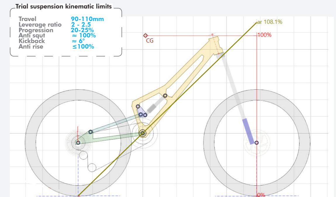
Figure 43. Final design in the sag position, developed with the use of the software linkage.
