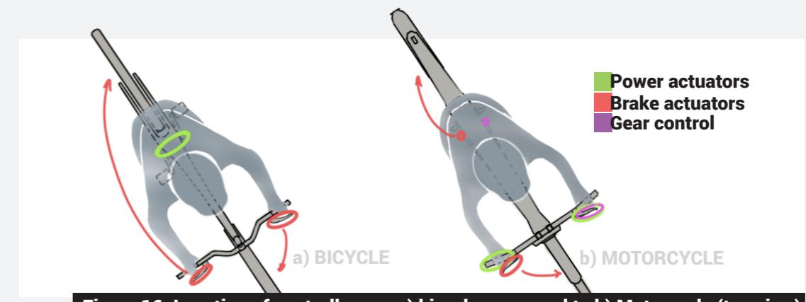
Figure 16. Location of controllers on a) bicycle compared to b) Motorcycle (top view)
