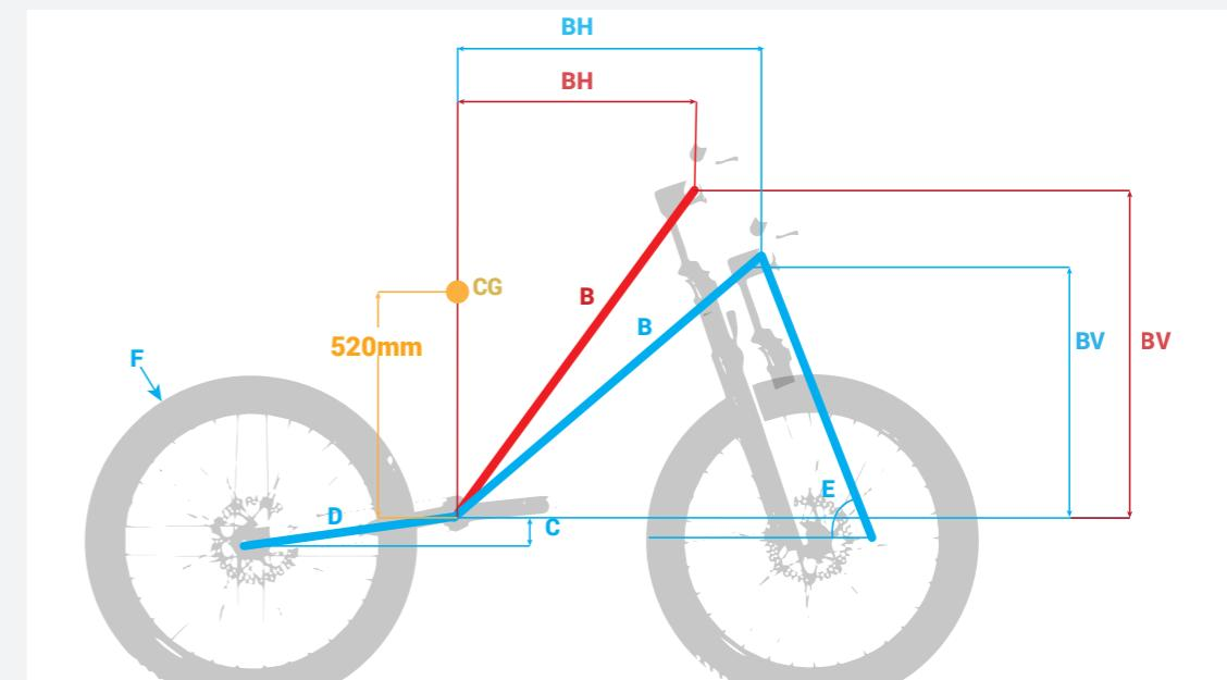
Figure 27. Dimensions required for a bike to behave like a trials bike, reach dimensions from the motorcycle, and height of the center of gravity.
