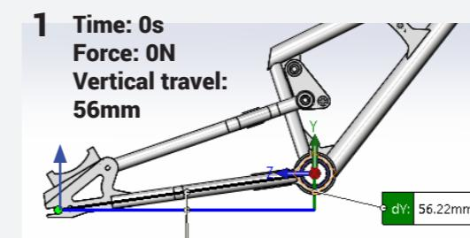
No weight is applied on the mechanism, therefore there is no rider on the bicycle.
