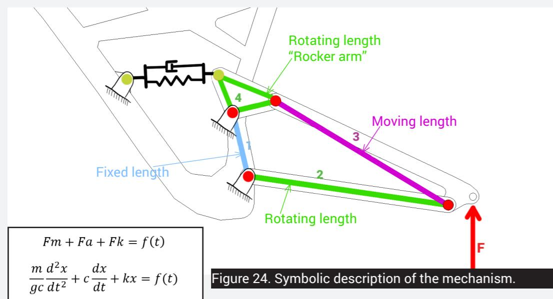
Figure 24. Symbolic description of the mechanism.
