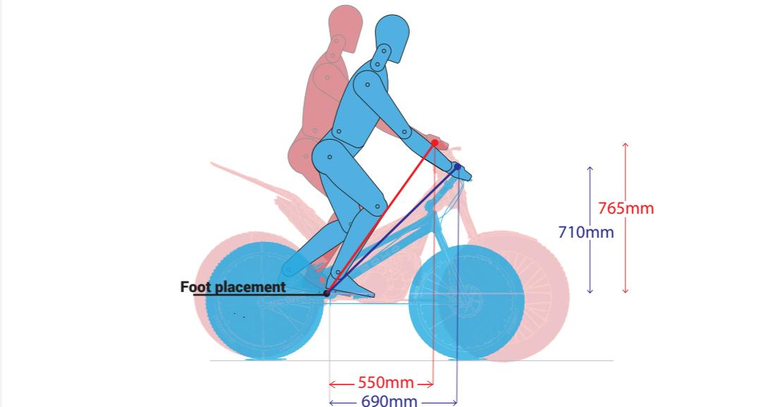
Figure 17. Reach on a bicycle compared to reach on a motorcycle and its influence on the posture
