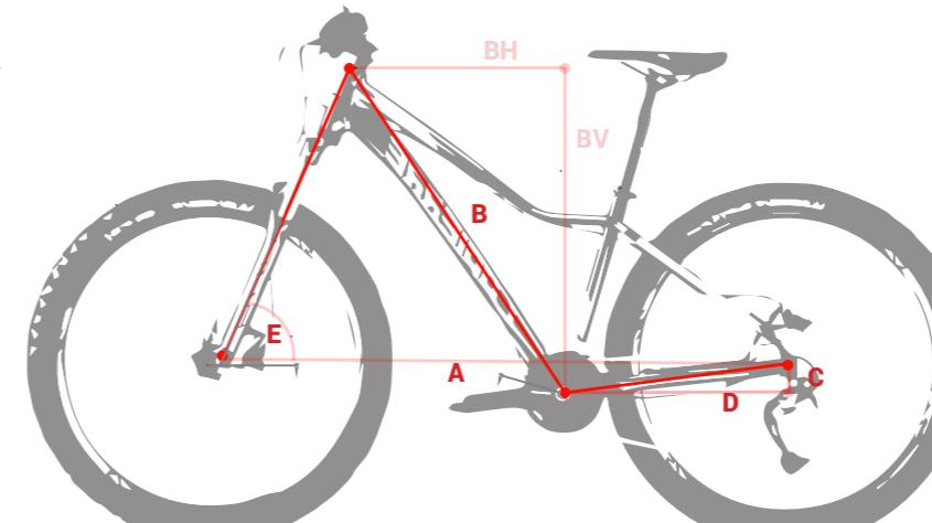
Figure 18. Frame geometry of trial bike compared to conventional bike (see average measurements in Table 3).
