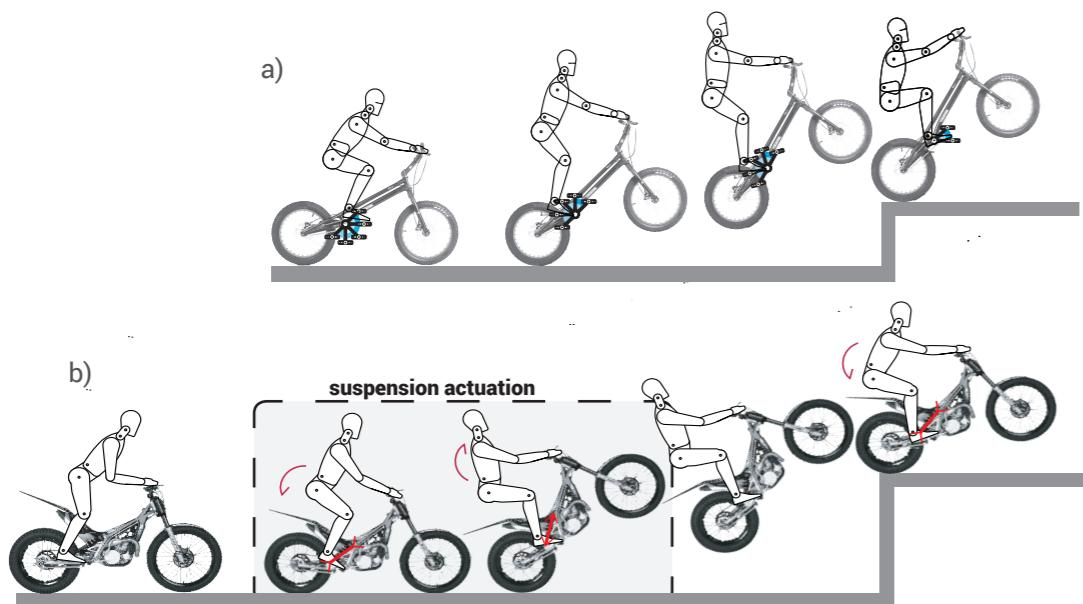
Figure 9. a) Climbing an obstacle with a bicycle. b) Climbing an obstacle with a motorcycle where suspension compression and body gesture are shown in red.
