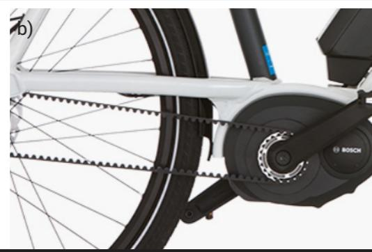
Figure 19. Electric bicycle systems. a)Hub motor , b) mid-drive motor.
