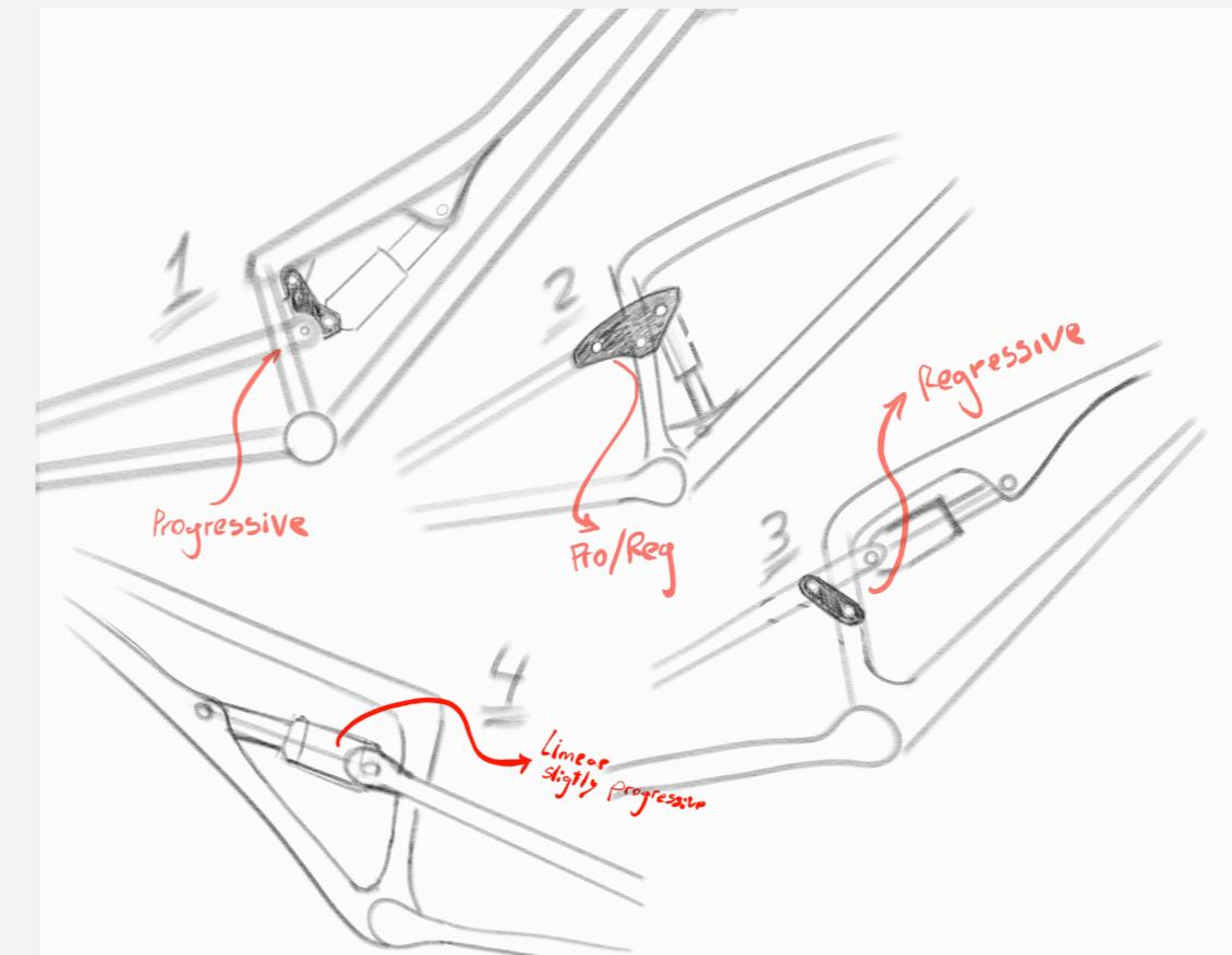
Figure 41. Configurations investigated and compared in terms of leverage ratio.
