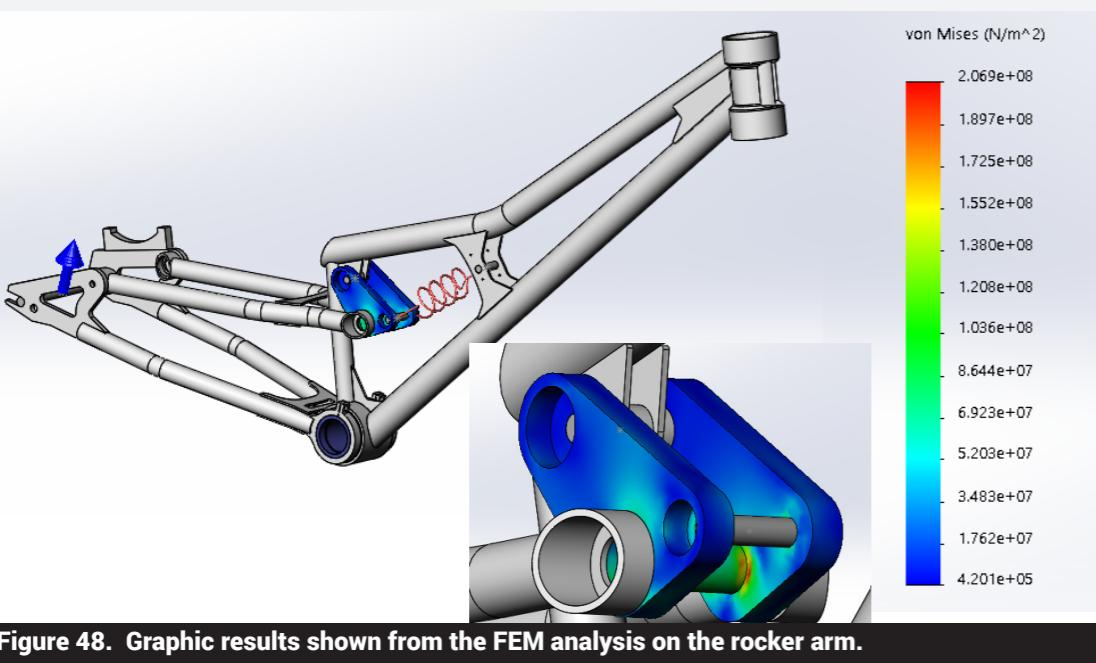
**Figure 48.** Graphic results shown from the FEM analysis on the rocker arm.
