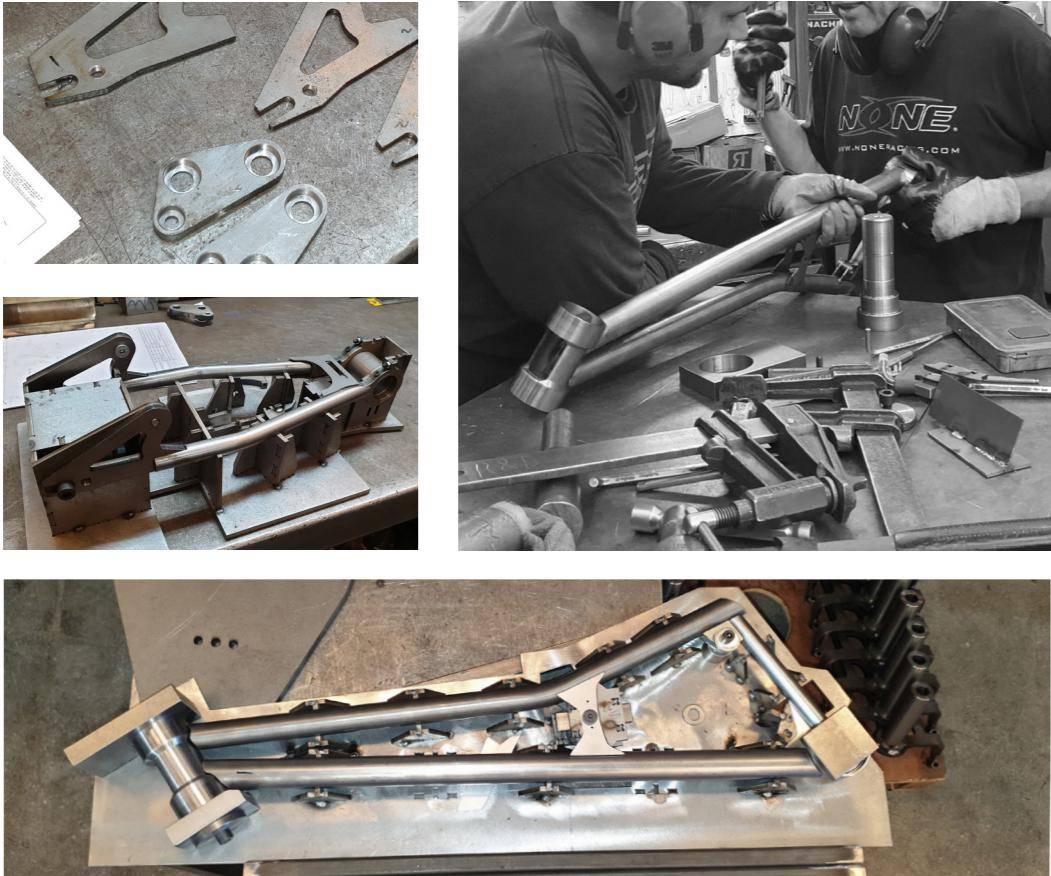
Figure 49. Photos taken during the assembly journey at the Dmotors factory (Engine derivatives).
