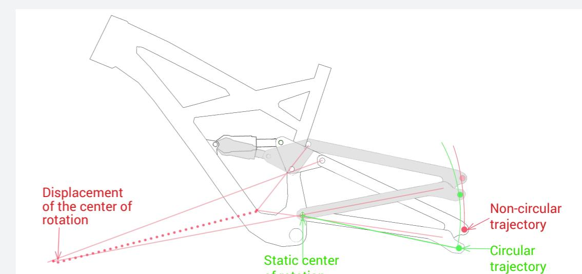
Figure 25. In green a system is described with a circular trajectory and in red a system with a non-circular trajectory.
