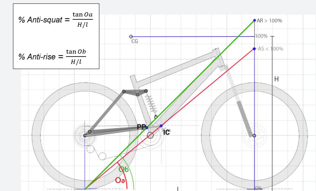
Figure 29. a) The red line goes through the instant center of rotation and is used to calculate anti-squat. b) The green line goes through the main pivot and is used to calculate anti-rise.
