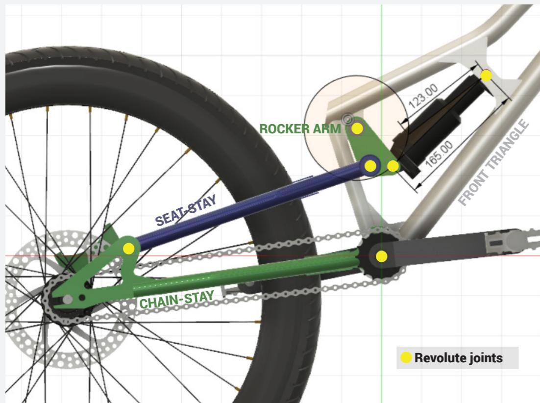
Figure 45. Complete 3D model naming each separate component of the frame.
