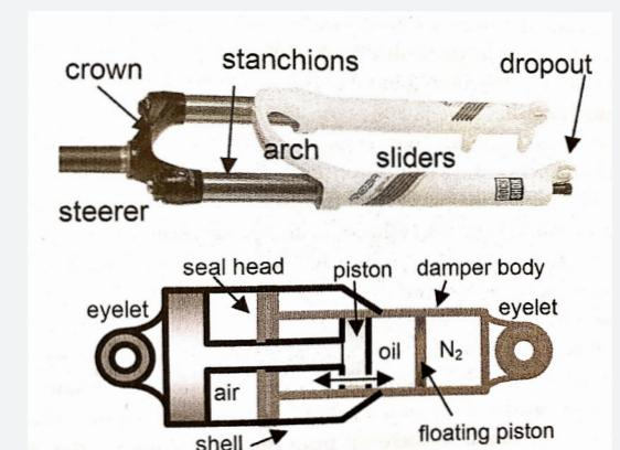
Figure 23. Schematic representation of fork and a rear shock.
