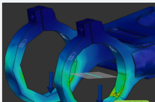
**Figure 47.** Graphic results shown from the FEM analysis on the chain-stay housing.
