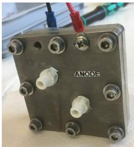
**Figure 10:** MEA cell after assembly. The blue and red wires are used for electrical connections
