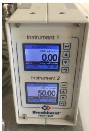
*Figure 12: Bronkhorst High-Tech Mass Flow Controller (MFC)*
