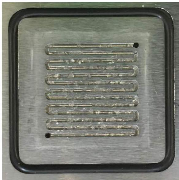
*Figure 24: Picture of the cathode-side gas flow channel after conducting CO<sub>2</sub>RR experiment at 200mA/cm<sup>2</sup> and 40 sccm. Large salt crystals are clearly visible*
