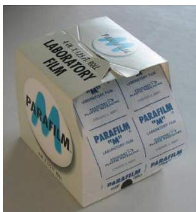
*Figure 13: PARAFILM Semi-transparent film used to cover anolyte container*
