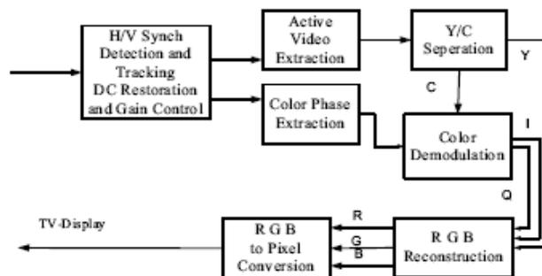
Fig. 2. Signal processing diagram of the NTSC receiver.
