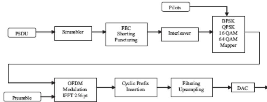
Fig. 3. WiMAX transmitter block diagram specified by the IEEE standard.
