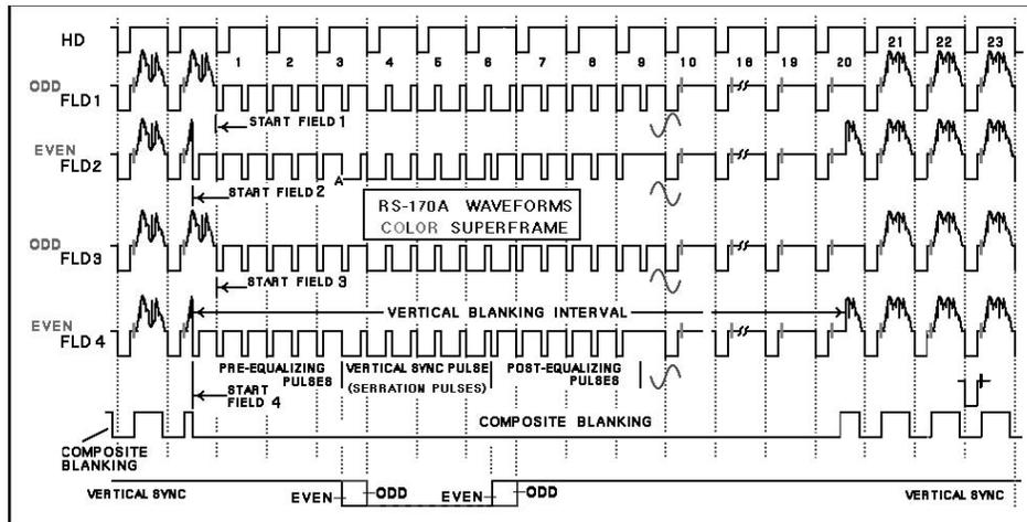
Fig. 1. Color field blanking sequence for NTC analog television system.
