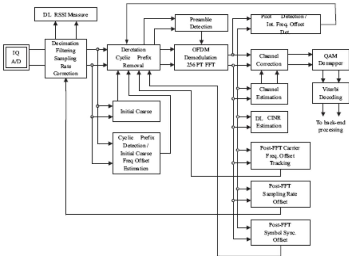
Fig. 4. WiMAX receiver signal processing blocks.
