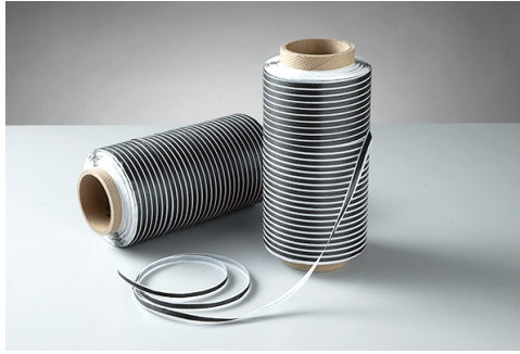
Figure 2.3: Spools of 1/4 inch carbon fibre prepreg material are shown, which can be used for fibre placement within an AFP process. The picture is from [24]
