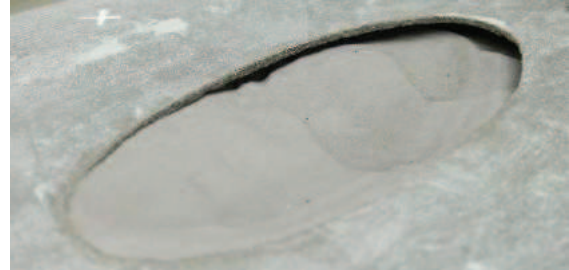
Figure 8. The developed scour hole in the water flume after 4 hours.
