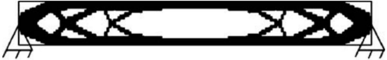
Figure 33: Results for the simply supported beam from Du and Olhoff [2007] with the use of a sensitivity filter.
