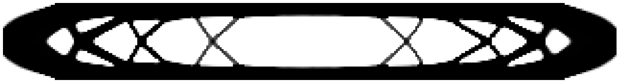
Figure 34: Results for the sensitivity filter with a filter radius of 3 elements.
