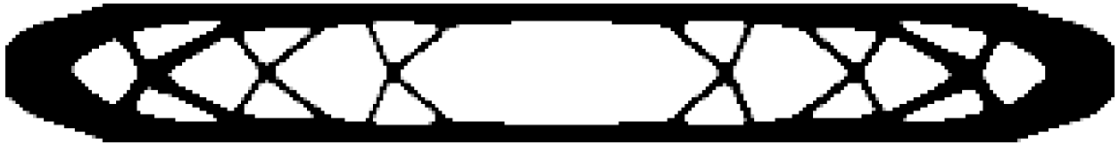
Figure 35: Level-set results of the CSRBF 4 and 6 elements support radius.
