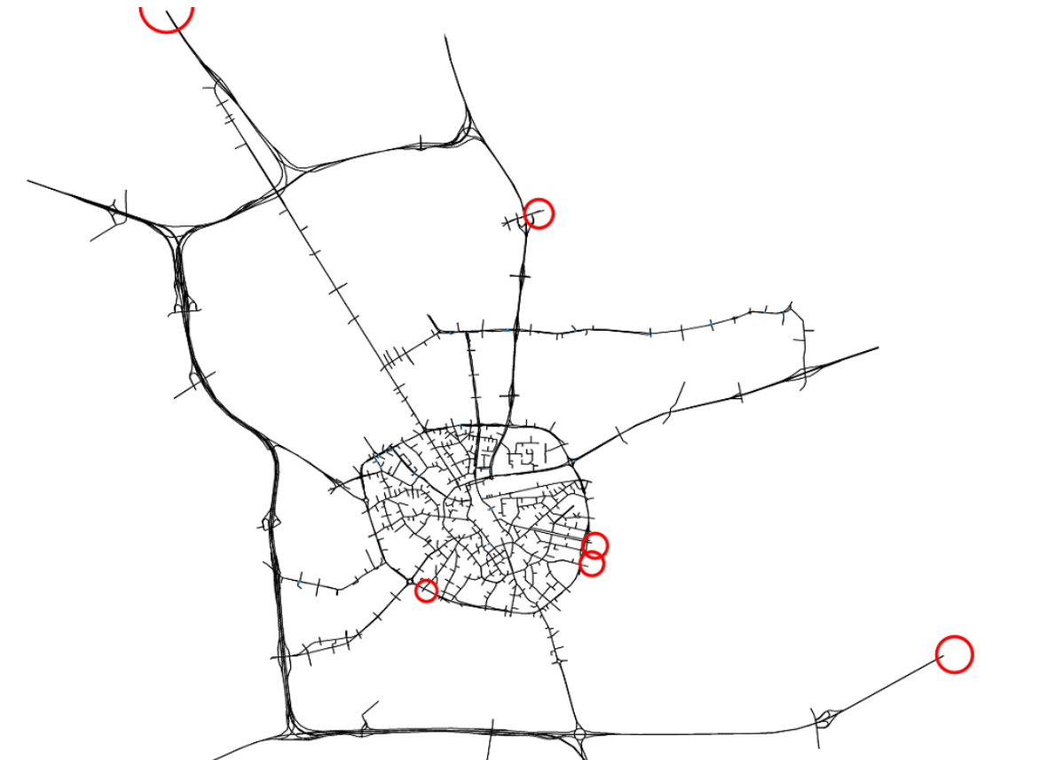
Figure 4.2: Test locations for testing if external zones generate the correct amount of traffic, for this check, the GEH statistic is used
