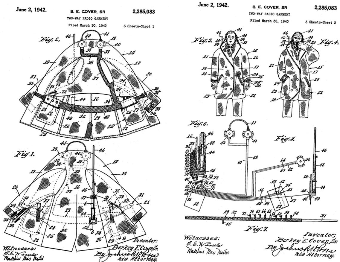
FIGURE 53.1 Cover (1942). Two-way radio garment, Patent N. US2285083A.
