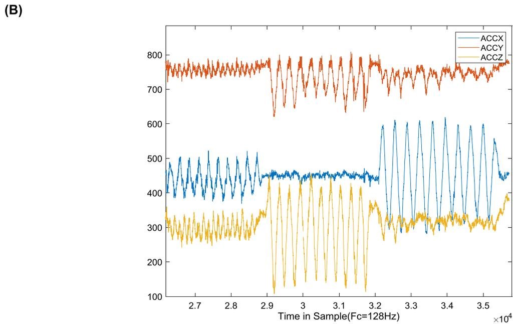
**FIGURE 53.10** An example of signal reliability protocol that consists of eight physical exercises recorded through a trunk-worn 3-axis accelerometer integrated into a smart clothing (A = all the protocol, B = three exercises (10 repetitions each)).
