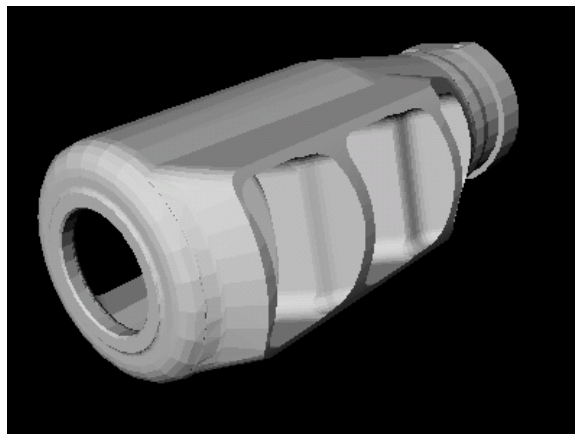
Figure 2: Three-chamber muzzle brake geometry, imported by GDT using CAD graphical format.
