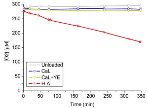
Figure 2: Oxygen concentration measurements on unloaded and loaded Liapor particles
