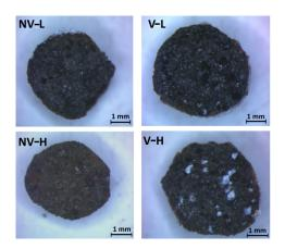
Figure 1: Liapor particles with different impregnation type
