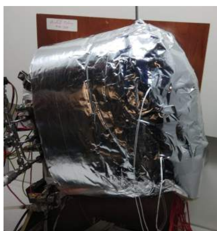
(a) Outer Rockwool insulation in the reactor
