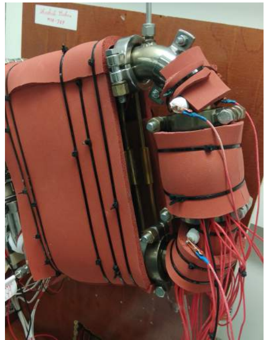
(b) The inner silicone sheet insulation for the reactor
