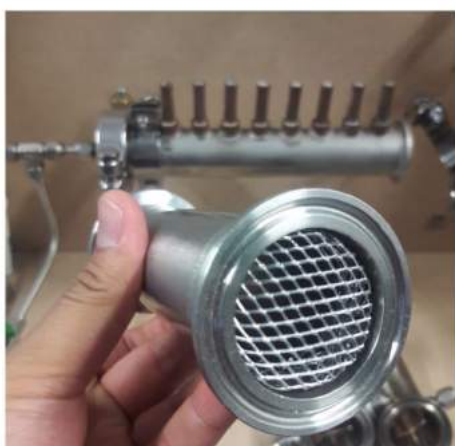
(a) The basket used for catalyst pellet support.
