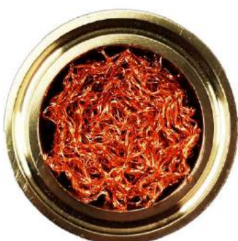
(a) The copper mesh inside the reactor pipe at heat pipe locations.
