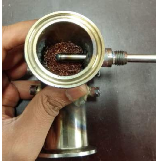
Figure E.5: The design of the thermowell well for gas flow temperature measurements.
