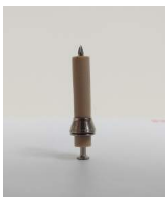
(a) PEEK and nail pass through fabrication.
