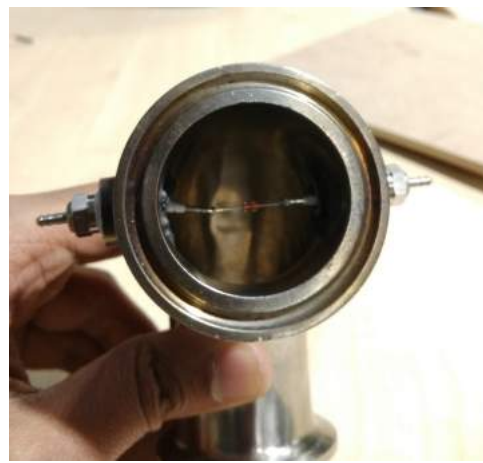
(b) The glow plug temperature sensor connection with reactor Tri-clamp pipe.
