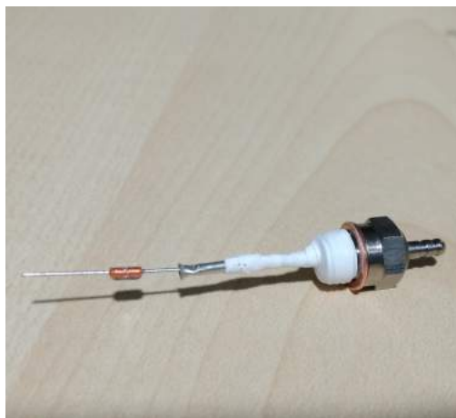
(a) The glow plug attachment to the temperature sensor.
