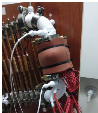
(b) PTFE & silicone pad insulation in the reactor hot section.
