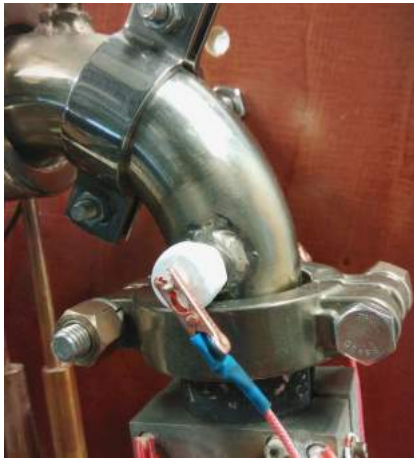
(a) The outside connection of the PEEK-Nail electrical pass-through.
