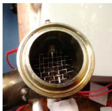
(b) Peek and nail pass through in the reactor Tri-Clamp pipe.
